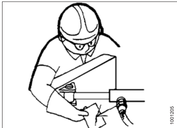
Figure 1.8: Testing for Hydraulic Leaks
