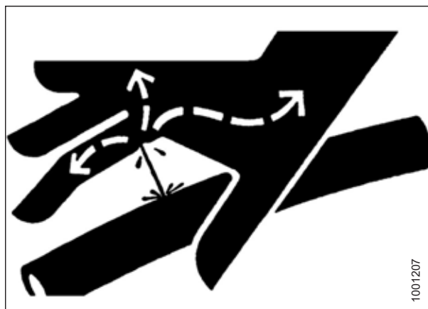
Figure 1.9: Hydraulic Pressure Hazard
