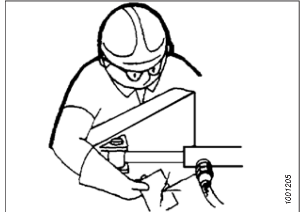
Figure 1.11: Test de fuites hydrauliques
