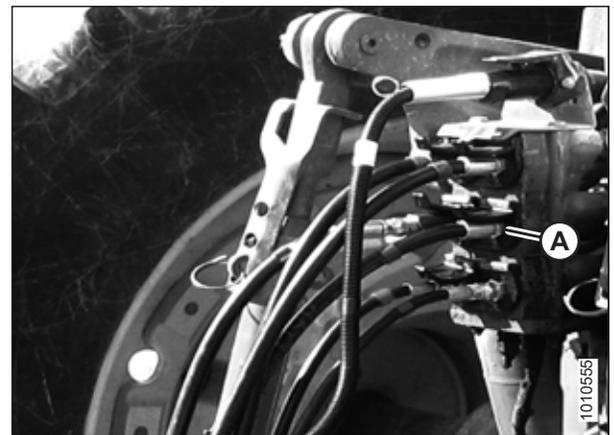
Figure 9.5: Raccord hydraulique
