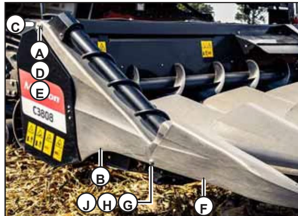
Figure 4.32: RED Installed on Header – Right Side
