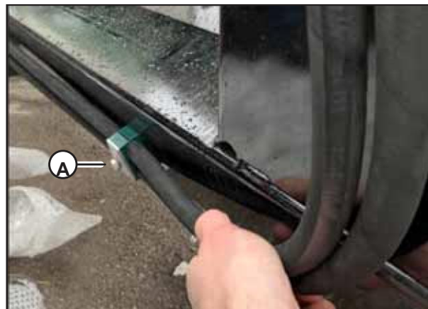
Figure 4.34: RED Hydraulic Hoses
