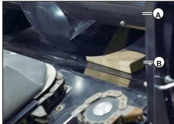
Figure 5.14: Auger Resting on Wood Block
