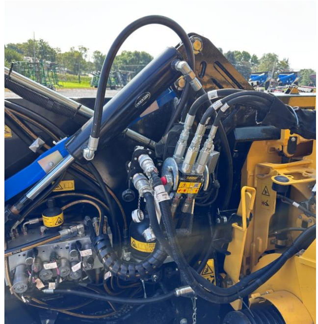
Figure 4.19: Multicoupler on a header Configured for a Case or New Holland Combine
