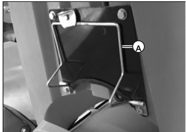
Figure 4.41: Wire Bracket Support Installed on Front Snout – Field Position
