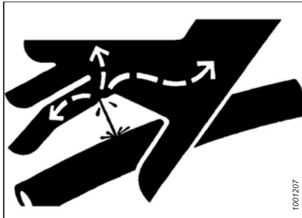
Figure 1.9: Hydraulic Pressure Hazard
