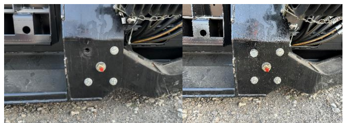
Figure 4.11: Reinstalling Bolt for Flex Linkage
