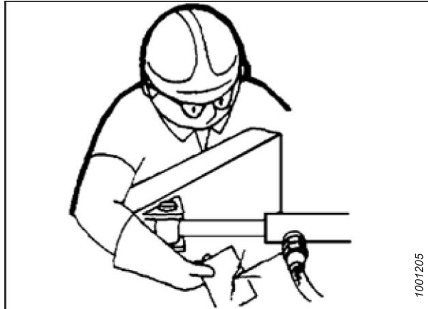
Figure 1.8: Testing for Hydraulic Leaks
