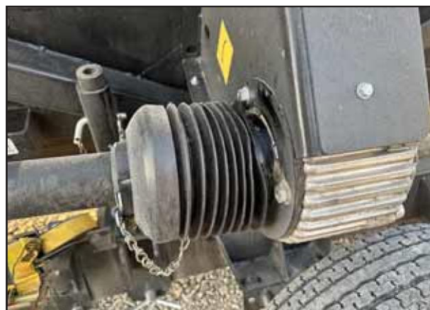
Figure 3.3: Main Driveline Guard – Incorrectly Seated
