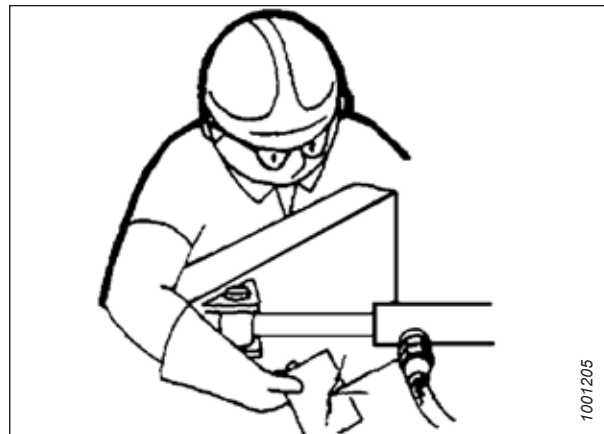
Figure 1.8: Testing for Hydraulic Leaks
