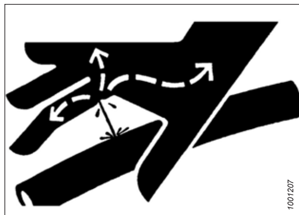
Figure 1.9: Hydraulic Pressure Hazard
