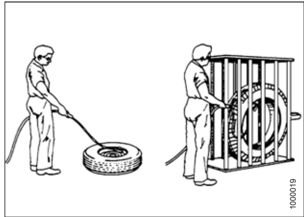
Figure 1.8: Safely Inflating Tire
