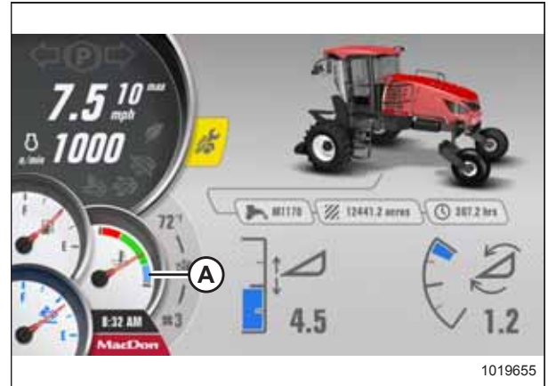
Figure 4.21: HPT No Header Screen
