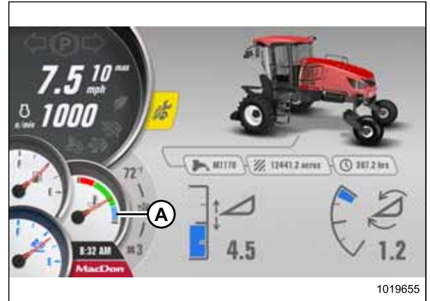
Figure 4.24: HPT No Header Screen
