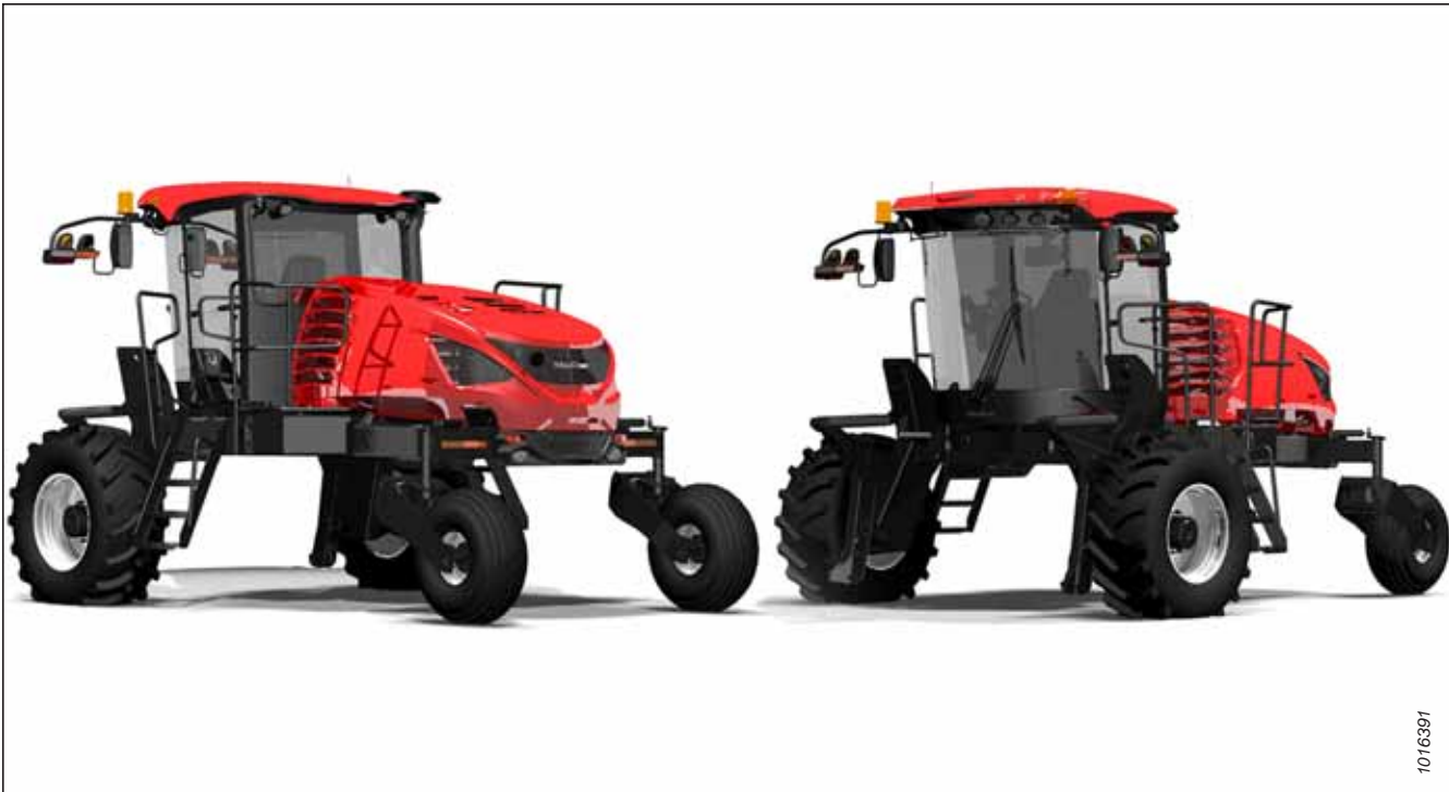
M1240 Windrower, featuring Dual Direction® and CrossFlex™ rear suspension
