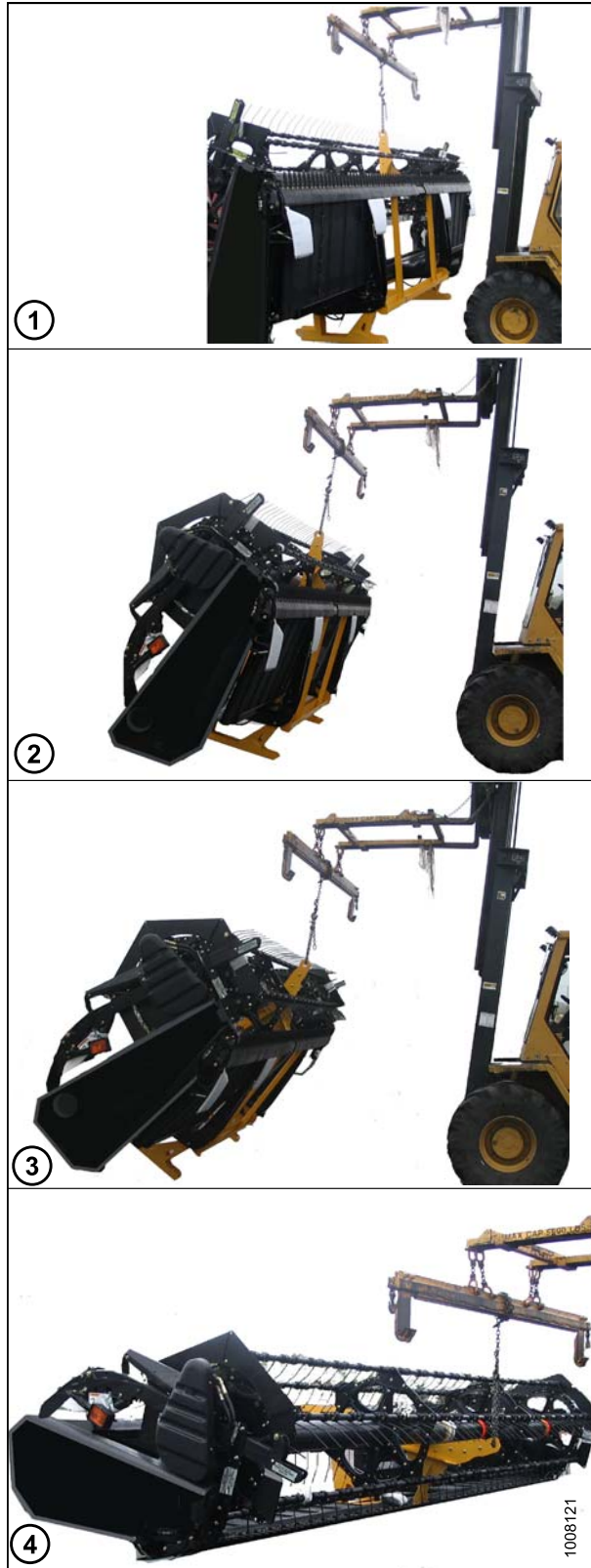
Figure 2.6: Lowering the Header
