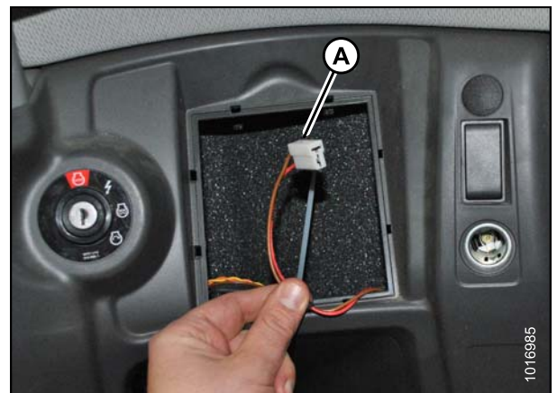
Figure 3.116: White Plug in Panel Beside Ignition
