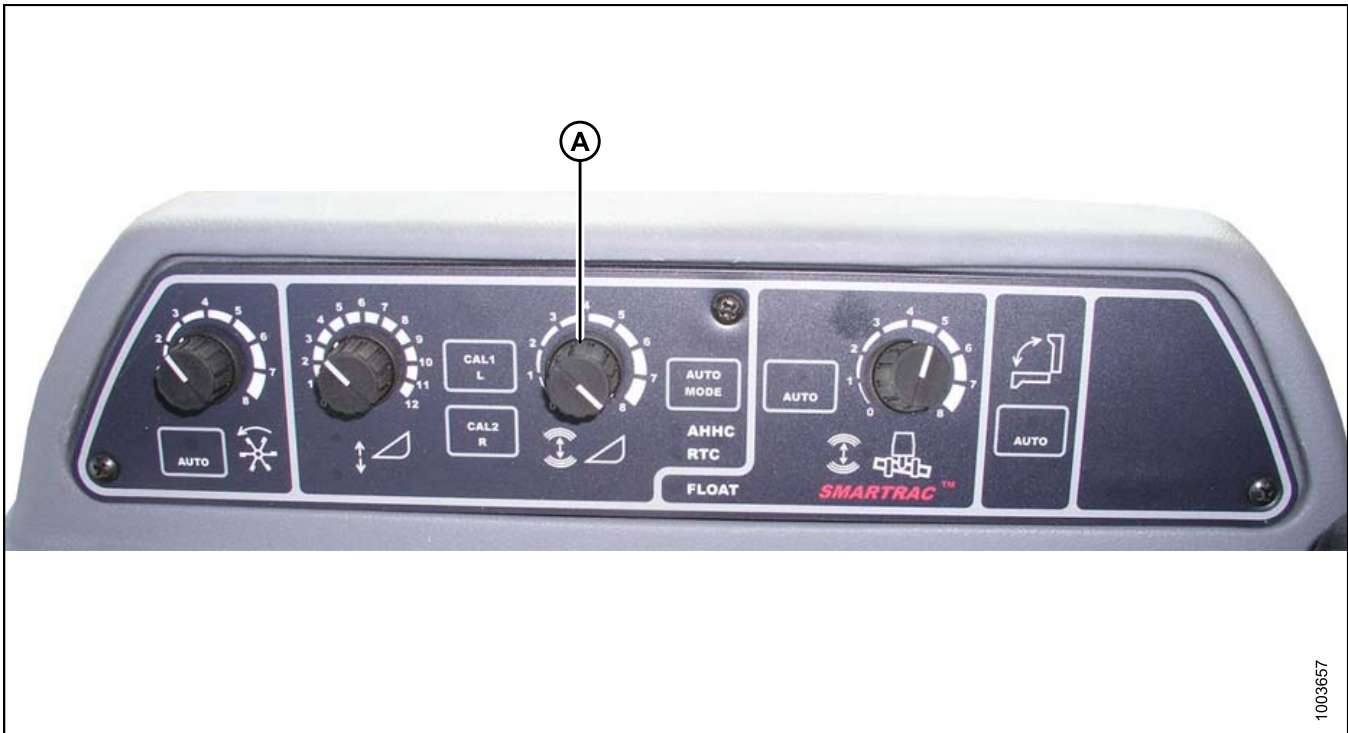
Figure 5.72: Auto Header Height Control (AHHC) Console
