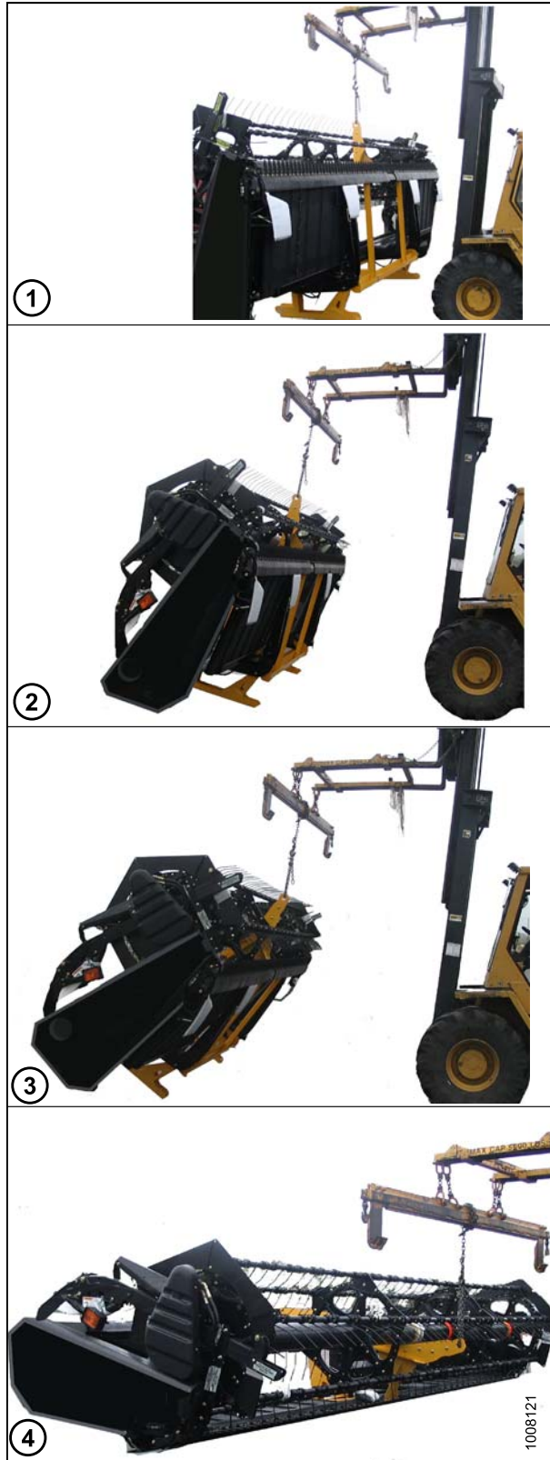
Figure 2.6: Lowering the Header
