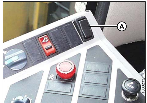
Figure 3.95: Rocker Switch in Place
