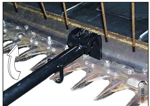
Figure 7.2: Guard Tips – Upward Adjustment
