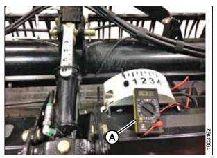
Figure 5.197: Float Indicator Reading 1 V
