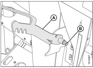
Figure 3.44: Feeder House Lever Lock on Adapter
