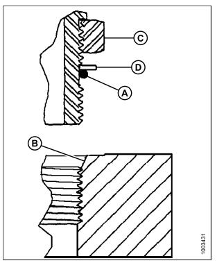
Figure 7.11: Hydraulic Fitting
