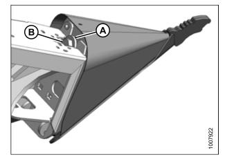
Figure 3.167: Crop Divider Installation
