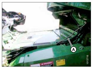
Figure 3.69: 60/70 Series Harness Routing
