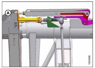
Figure 4.62: Wing Lock in Lock Position
