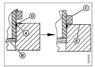
Figure 7.12: Hydraulic Fitting
