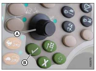
Figure 5.160: John Deere Combine Control Console A - Scroll Knob B - Check Mark Button
