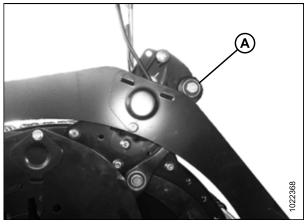
Figure 3.154: Right Reel with Cam Arms Attached
