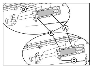
Figure 4.67: Feed Draper Tensioner (Spring Box Drawn Transparent)
