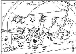
Figure 5.7: Most Common 5 Volt AHHC Sensor Assembly
