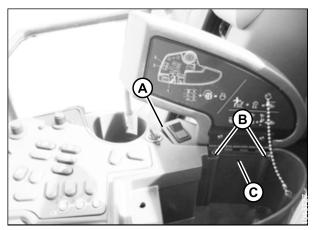
Figure 3.76: Switch Plate Mounting
