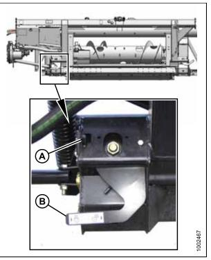
Figure 3.150: Float Lock in UNLOCK Position
