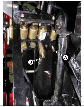
Figure 5.77: Header Raise and Lower Adjustable Restrictors
