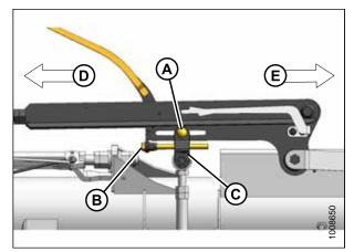
Figure 4.61: Balance Linkage
