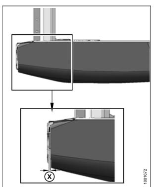
Figure 4.84: Gap Between Endshield and Header Frame
