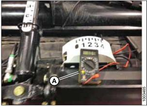
Figure 5.198: Float Indicator Reading 4.3 V
