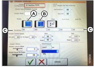
Figure 5.97: Automatic Controls and Sensitivity Settings
