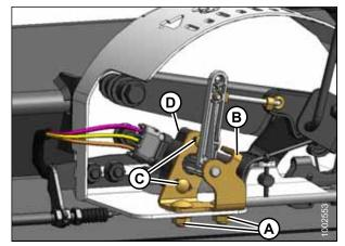
Figure 5.123: AHHC Sensor AssemblyA - Sensor Support Mounting BoltsB - Sensor SupportC - Sensor Mounting BoltsD - Potentiometer
