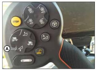
Figure 5.104: Header Down Switch
