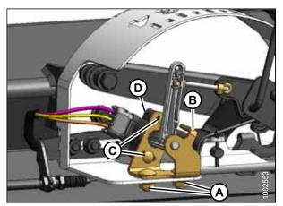
Figure 5.199: AHHC Sensor Assembly
