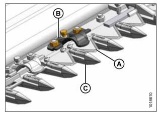
Figure 4.9: Normal Guard Hold-Down
