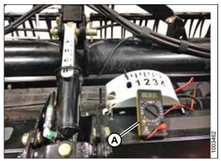
Figure 5.4: Measuring Voltage at Float Indicator Box
