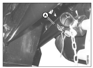
Figure 3.155: Shipping Wire and Brace
