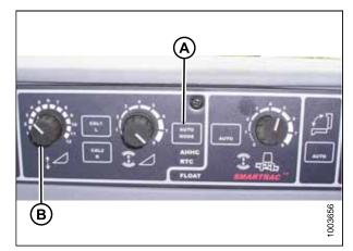
Figure 5.78: Auto Header Height Control Console
