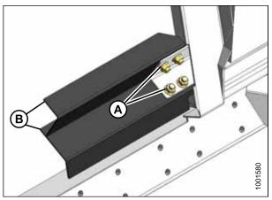
Figure 3.20: Auger Stripper Bar
