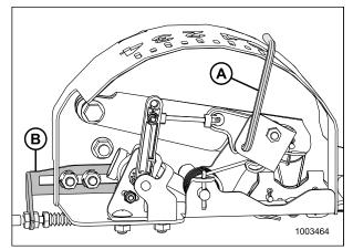
Figure 5.48: Float Indicator Box (Most Common 5 Volt AHHC Sensor Assembly Shown)
