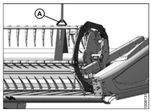
Figure 3.6: Left End Reel Lift
