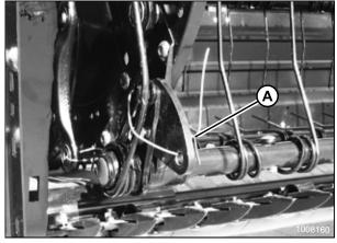
Figure 3.151: Disconnected Cam Links and Shipping Wire
