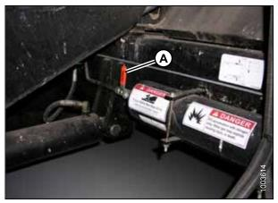
Figure 5.76: Combine Accumulator ON/OFF Switch A - Accumulator Lever (Off Position)
