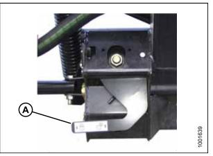
Figure 4.31: Header Float Lock in Unlock Position
