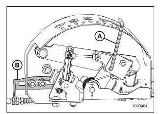
Figure 5.19: Float Indicator Box (Most Common 5 Volt AHHC Sensor Assembly Shown)
