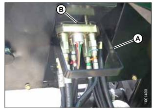
Figure 3.79: Multicoupler Storage
