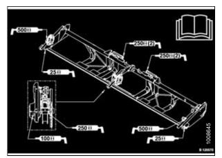
Figure 4.77: FD75 Master Grease Point Decal
