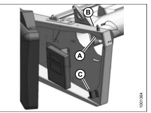
Figure 4.85: Endshield Adjustment
