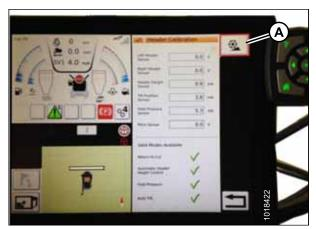
Figure 5.105: Header Calibration
