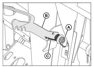
Figure 3.45: Feeder House Lever Lock on Adapter
