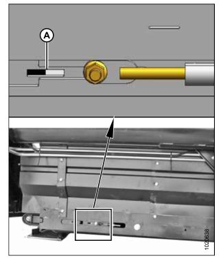
Figure 4.69: Tension Adjuster (Left Shown – Right Opposite)
