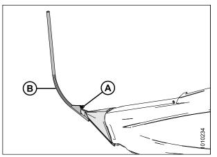
Figure 3.174: Divider Rod on Crop Divider
