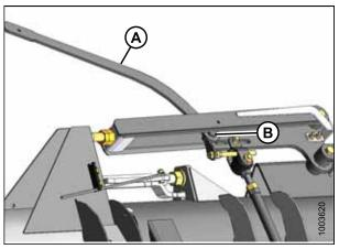
Figure 4.45: Balance Linkage
