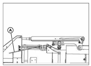
Figure 4.57: Wing Lock in UNLOCK Position
