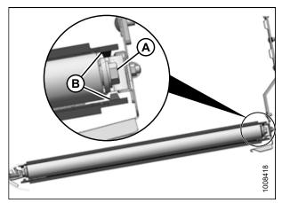
Figure 4.71: Idler Roller – Typical Both Ends of Roller
