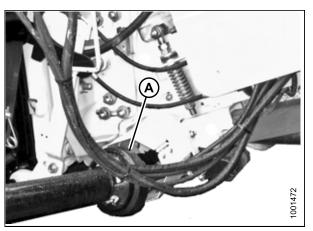
Figure 3.149: Driveline and Output Shaft
