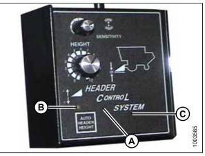
Figure 5.64: Combine Header Control System
