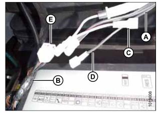
Figure 3.114: Power Source Connection
