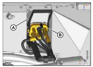
Figure 3.37: Adapter Multicoupler
