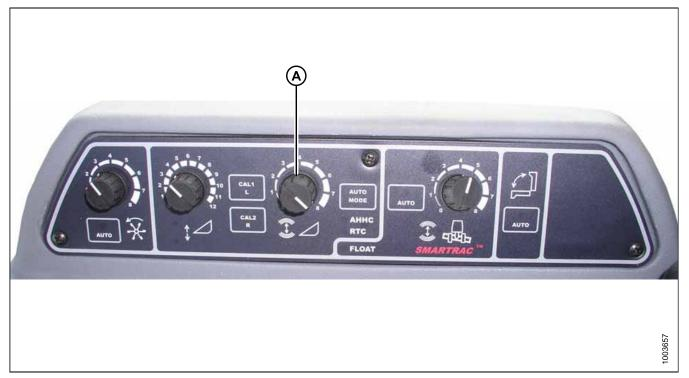
The SENSITIVITY ADJUSTMENT dial (A) controls the distance cutterbar must travel up or down before AHHC reacts and raises or lowers feeder house.
