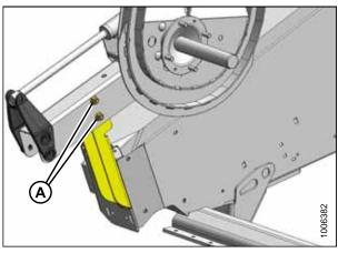
Figure 3.1: Reel Outboard Support Arm
