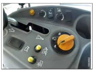
Figure 5.58: Height Adjustment Knob on Combine Control Console
