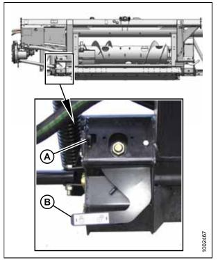
Figure 3.137: Float Lock in UNLOCK Position
