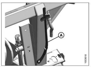
Figure 4.58: Torque Wrench
