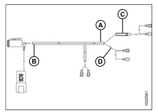
Figure 3.86: MD #279753 Wiring Harness
