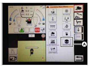
Figure 5.109: Direct Calibration Menu
