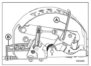
Figure 5.166: Float Indicator Box (Most Common 5 Volt AHHC Sensor Assembly Shown)
