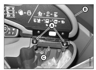
Figure 3.62: Support Position on Console
