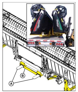
Figure 2.2: Header Shipping Supports
