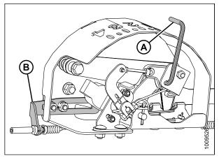
Figure 5.271: 10 Volt AHHC Sensor Assembly
