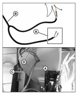
Figure 3.107: Switch Harness Connection
