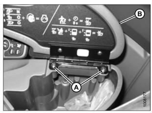
Figure 3.59: Storage Compartment and Cover
