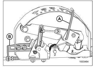
Figure 5.220: Float Indicator with Auto Header Height Sensor
