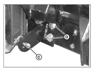
Figure 3.81: Feeder House Pin
