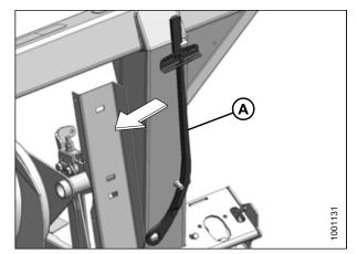
Figure 4.33: Torque Wrench
