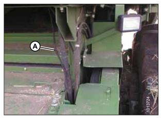
Figure 3.71: Switch Harness Routing
