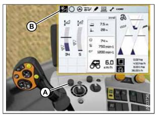
Figure 5.235: CLAAS Combine Display, Console, and Joystick
