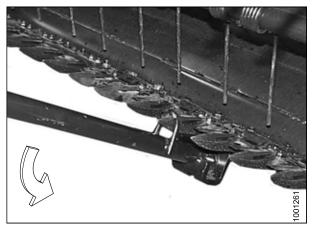
Figure 6.9: Guard Tips – Downward Adjustment
