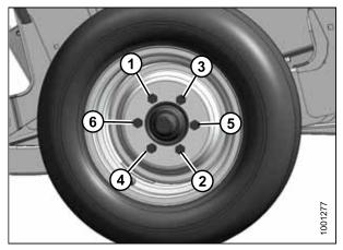
Figure 4.1: Bolt Tightening Sequence
