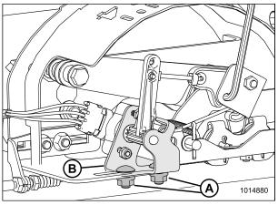
Figure 5.6: AHHC Sensor Assembly for Use with Lexion Combines
