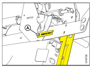
Figure 3.10: Reel Right Arm (Parts Removed for Clarity)
