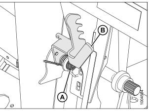
Figure 3.43: Feeder House Lever Lock on Adapter
