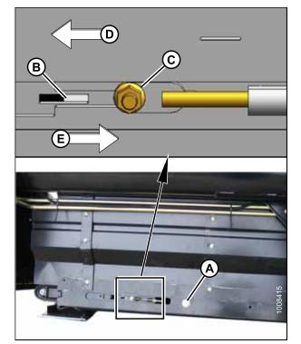
Figure 4.72: Tension Adjuster (Left Shown – Right Opposite)
