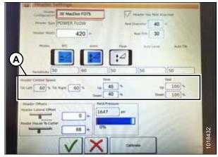
Figure 5.98: Header Speed Control Settings
