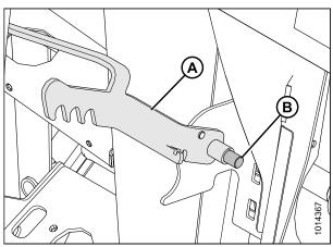
Figure 3.139: Feeder House Lever Lock on CA25
