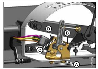
Figure 5.223: AHHC Sensor Assembly
