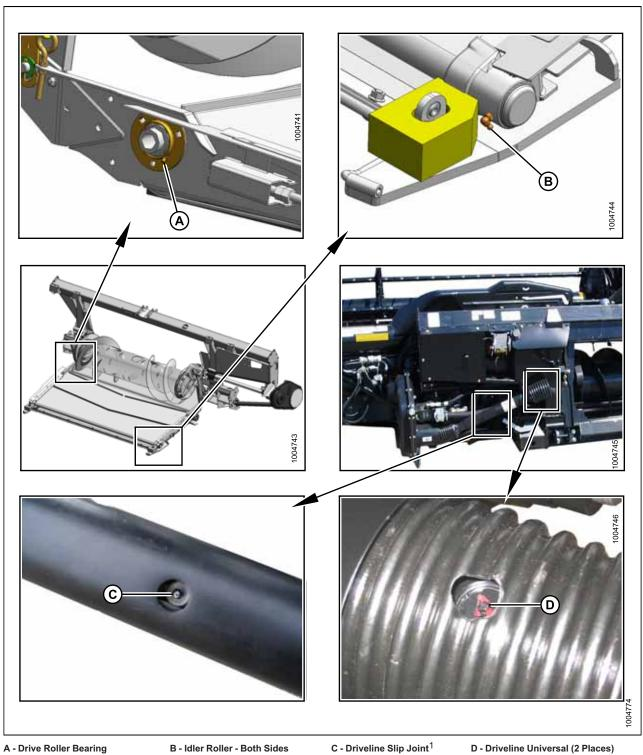
Figure 4.80: Drive Roller Bearing, Idler Roller, Slip Joint, and Driveline Universal
