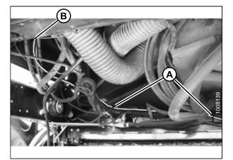
Figure 3.27: Harness under Right Side of Cab Floor
