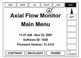
Select SUB SYSTEM (A). The SUB SYSTEM page displays. Figure 5.20: Case 8010 Combine Display
