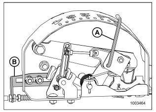
Figure 5.196: Float Indicator with Auto Header Height Sensor
