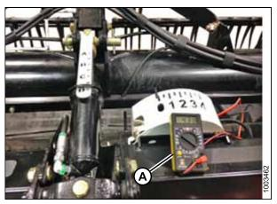
Figure 5.221: Float Indicator Reading 1 V
