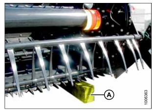
Figure 2.7: Blocks at Each End of Cutterbar
