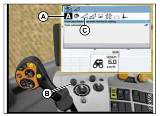
Figure 5.226: CLAAS Combine Display, Console, and Joystick
