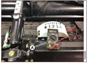
Figure 5.119: Checking Voltage with Voltmeter
