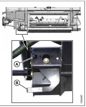
Figure 3.85: Float Lock in UNLOCK Position
