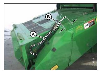
Figure 3.68: 50 Series Harness Routing
