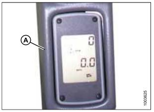
Figure 5.81: Tachometer
