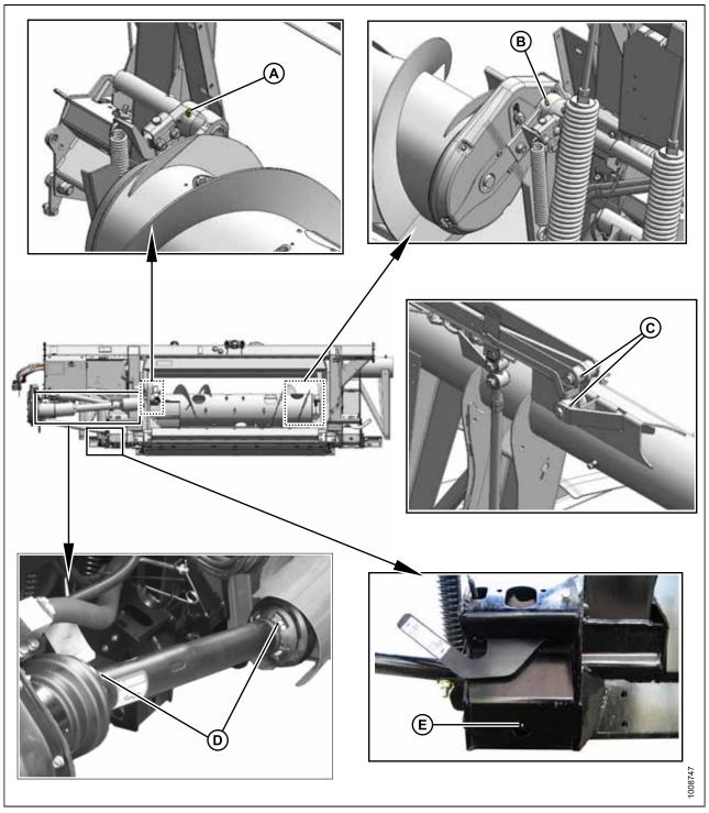
Figure 4.81: Float Pivot, Driveline Guard, Flex Linkage, and Auger Pivot
