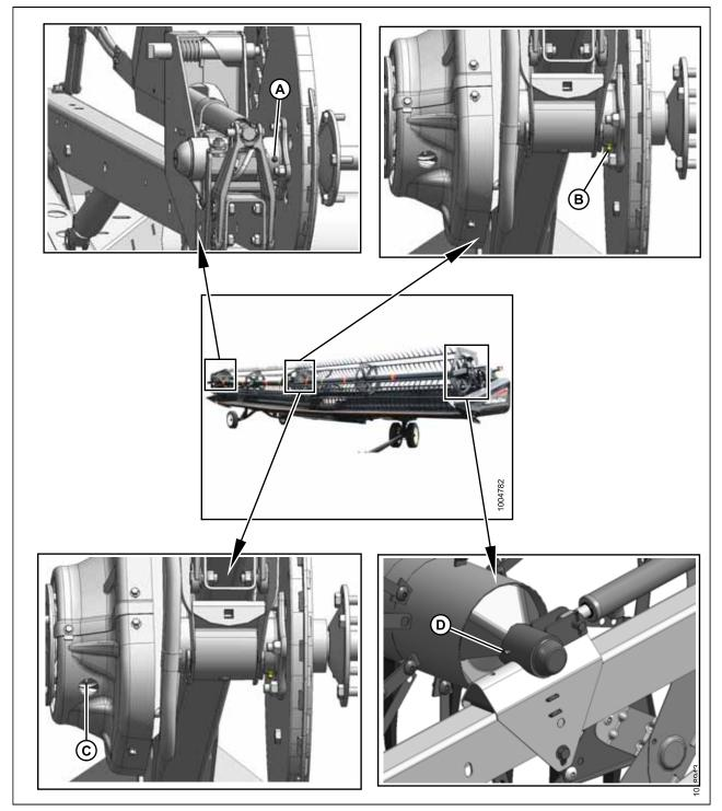
A - Reel Shaft Right Bearing (1 Place) D - Reel Shaft Left Bearing (1 Place)
