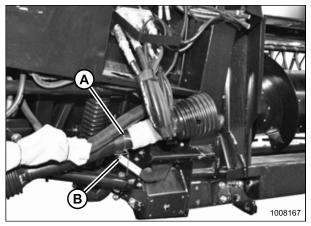
Figure 3.147: Shipping Wire on Driveline and Float Lock Lever
