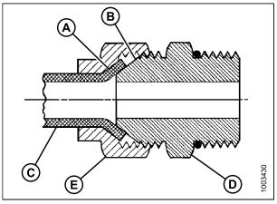
Figure 7.10: Hydraulic Fitting
