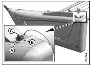
Figure 3.173: Left Endshield Pin
