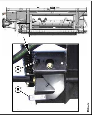
Figure 3.58: Float Lock in UNLOCK Position
