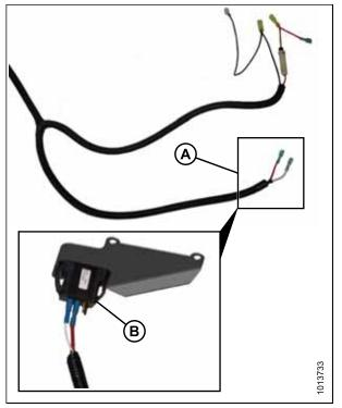
Figure 3.75: Switch End of Harness and Switch
