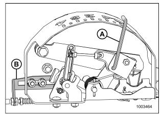
Figure 5.151: Float Indicator Box (Most Common 5 Volt AHHC Sensor Assembly Shown)
