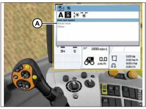
Figure 5.237: CLAAS Combine Display, Console, and Joystick
