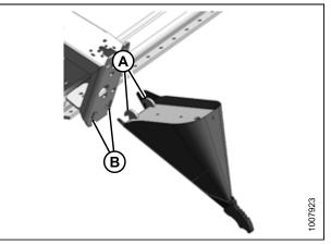
Figure 3.166: Crop Divider Installation
