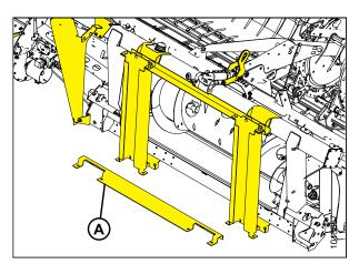
Figure 2.9: Lower Brace Removal
