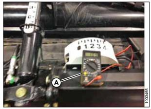
Figure 5.222: Float Indicator Reading 4.3 V
