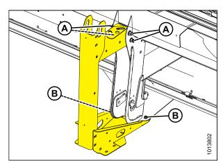
Figure 2.14: Shipping Stands at Outboard Header Legs (Right Side Shown)
