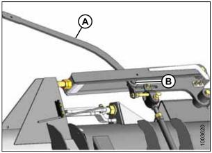
Figure 4.59: Balance Linkage
