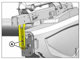
Figure 3.9: Reel Outboard Arm Support
