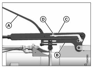
Figure 4.46: Balance Linkage
