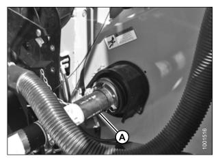
Figure 3.136: Driveline and Output Shaft
