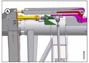
Figure 4.52: Wing Lock in Lock Position
