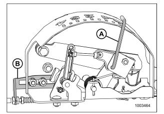
Figure 5.117: Float Indicator Box with Auto Header Height Sensor
