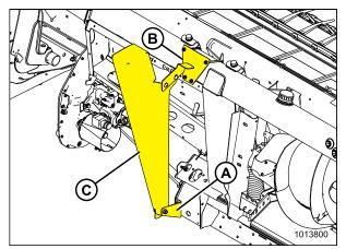
Figure 2.13: Multicoupler Guard
