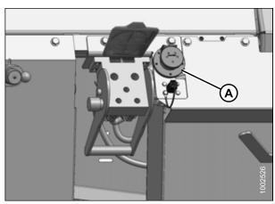
Figure 3.52: Electrical Receptacle
