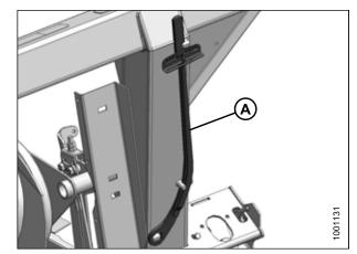
Figure 4.38: Torque Wrench
