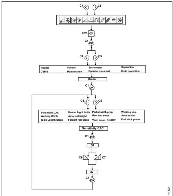
Figure 5.211: Flow Chart for Setting Sensitivity of Float Optimizer
