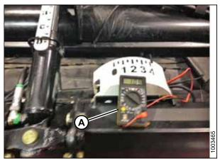
Figure 5.5: Measuring Voltage at Float Indicator Box
