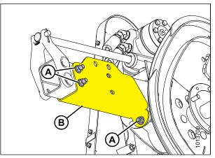
Figure 3.12: Reel Center Arm Shipping Channel
