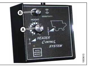
Figure 5.69: Combine Header Control System
