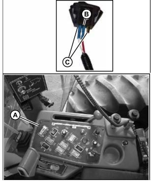
Figure 3.30: Switch and Console
