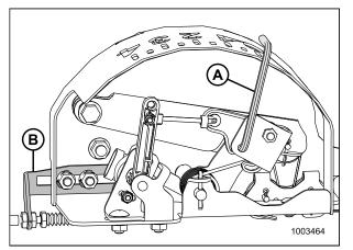
Figure 5.270: Float Indicator Box (Most Common 5 Volt AHHC Sensor Assembly Shown)
