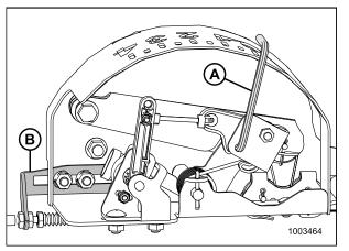
Figure 5.121: Float Indicator Box with Auto Header Height Sensor
