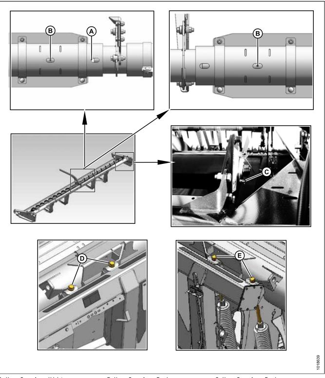
Figure 4.79: Upper Cross Auger and Float Spring Tensioners
