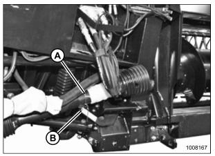
Figure 3.55: Shipping Wire on Driveline and Float Lock Lever
