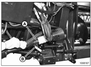
Figure 3.40: Adapter Shipping Configuration
