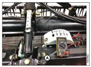
Figure 5.118: Checking Voltage with Voltmeter
