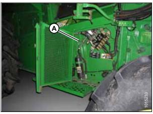
Figure 5.130: Accumulator Shut-off
