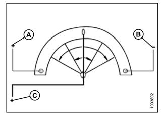
Figure 5.288: Power, Ground, and Signal Wires
