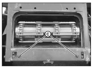
Figure 3.34: AGCO Group Alignment Pins
