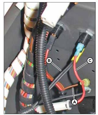
Figure 3.99: Two Connector Hookup: Switch Harness Installed
