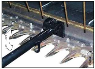
Figure 6.8: Guard Tips – Upward Adjustment
