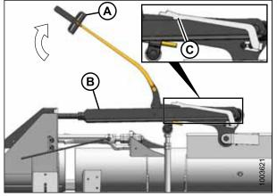
Figure 4.47: Balance Linkage
