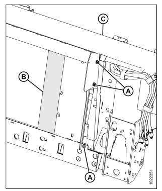
Figure 3.31: Filler Plate on Right Side of Transition Frame
