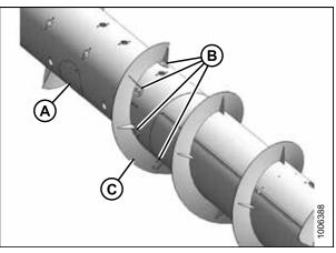
Figure 3.19: Auger Flighting Extension
