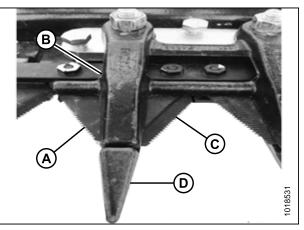
Figure 4.10: Double-Knife Center Guard Hold-Down
