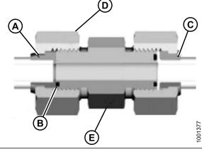
Figure 7.15: Hydraulic Fitting
