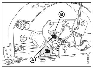
Figure 5.8: 10 Volt AHHC Sensor Assembly for Use with Some New Holland Combines
