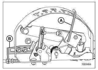
Figure 5.140: Float Indicator Box (Most Common 5 Volt AHHC Sensor Assembly Shown)
