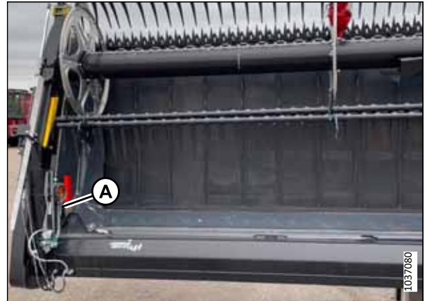
Figure 2.8: Parts Secured to Header
