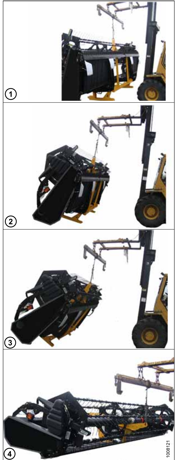
Figure 2.19: Lowering Header to the Ground
