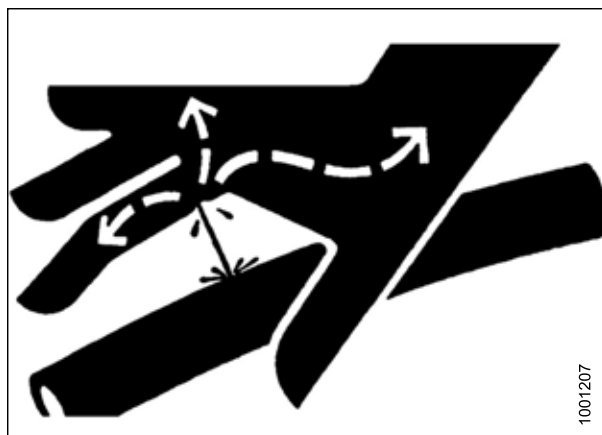
Figure 1.9: Hydraulic Pressure Hazard
