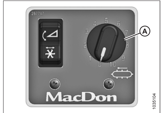
Figure 10.5: In-Cab Side Draper Speed Control – IDEAL™, Challenger®, CLAAS, Gleaner®, John Deere, and Massey Ferguson® Combines
