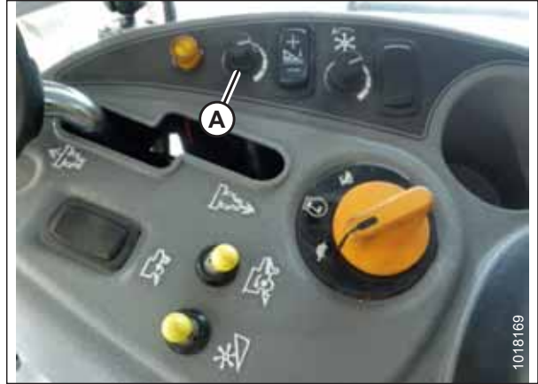
Figure 8.104: Height Adjustment Knob on the Combine Control Console
