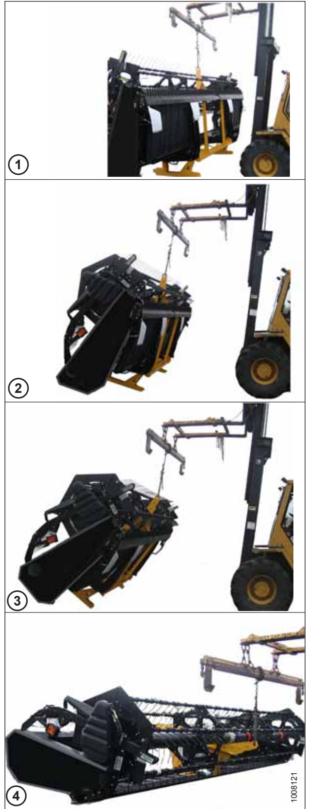
Figure 2.6: Header Lowered onto Ground
