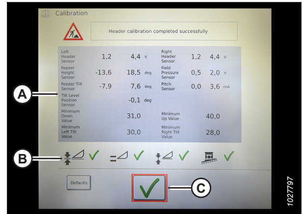
Figure 7.282: Completed Calibration Page
