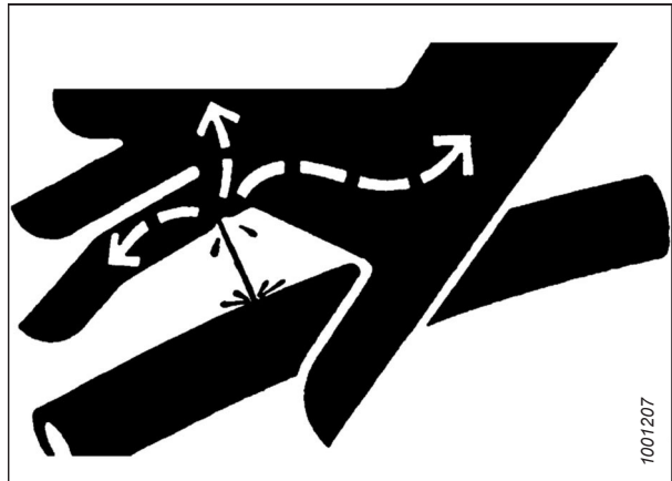
Figure 1.12: Hydraulic Pressure Hazard
