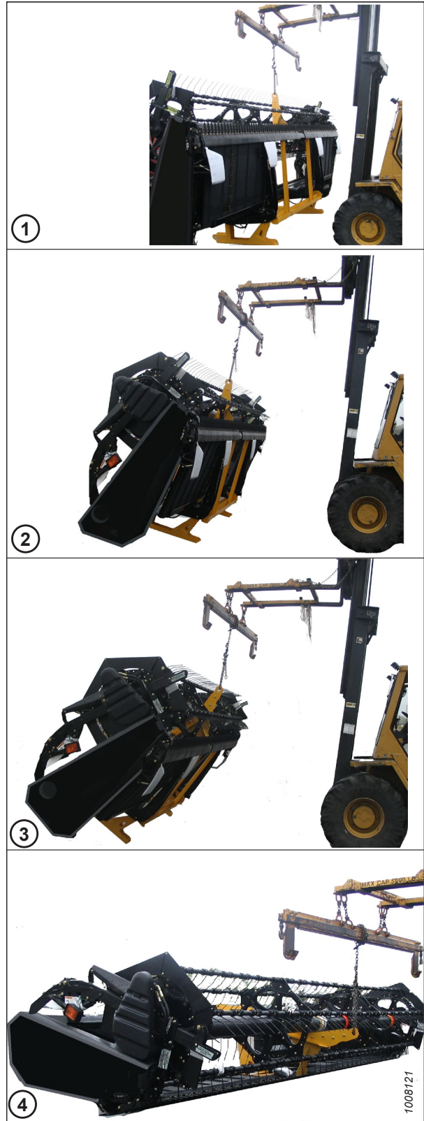
Figure 2.5: Header Lowered onto Ground
