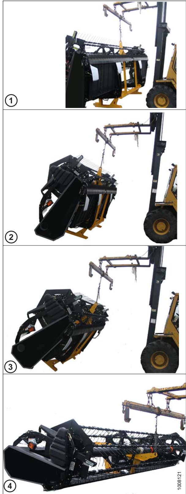
Figure 2.6: Header Lowered onto Ground
