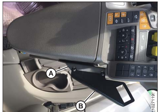
Figure 5.70: Top View of Armrest Showing Supports Installed in Preferred Location
