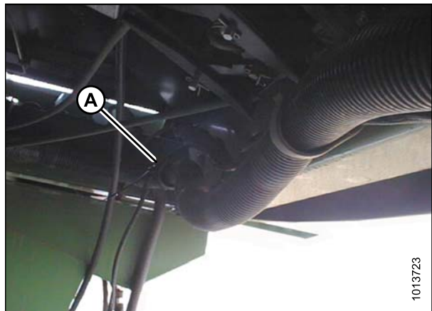
Figure 5.49: Switch Harness Routing
