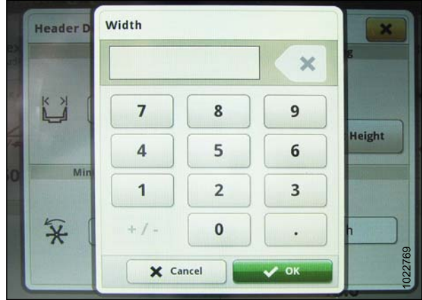
Figure 7.280: John Deere S7 Display – Setting Header Width
