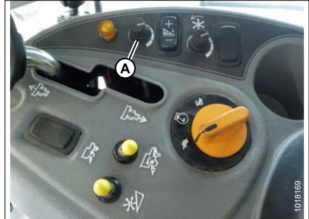
Figure 7.108: Height Adjustment Knob on the Combine Control Console
