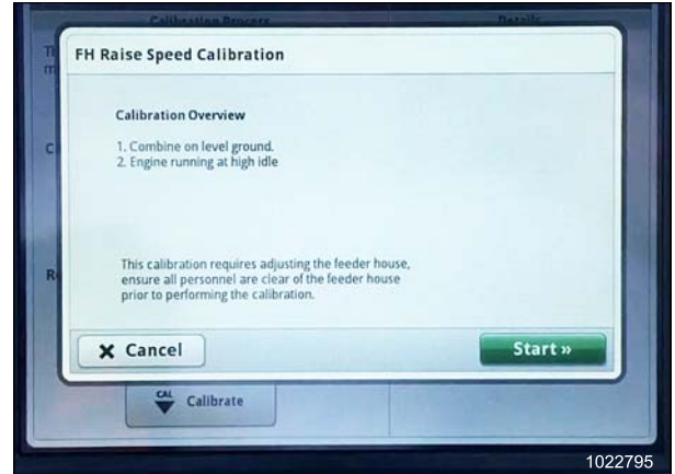
Figure 7.297: John Deere S7 Display – Feeder House Calibration
