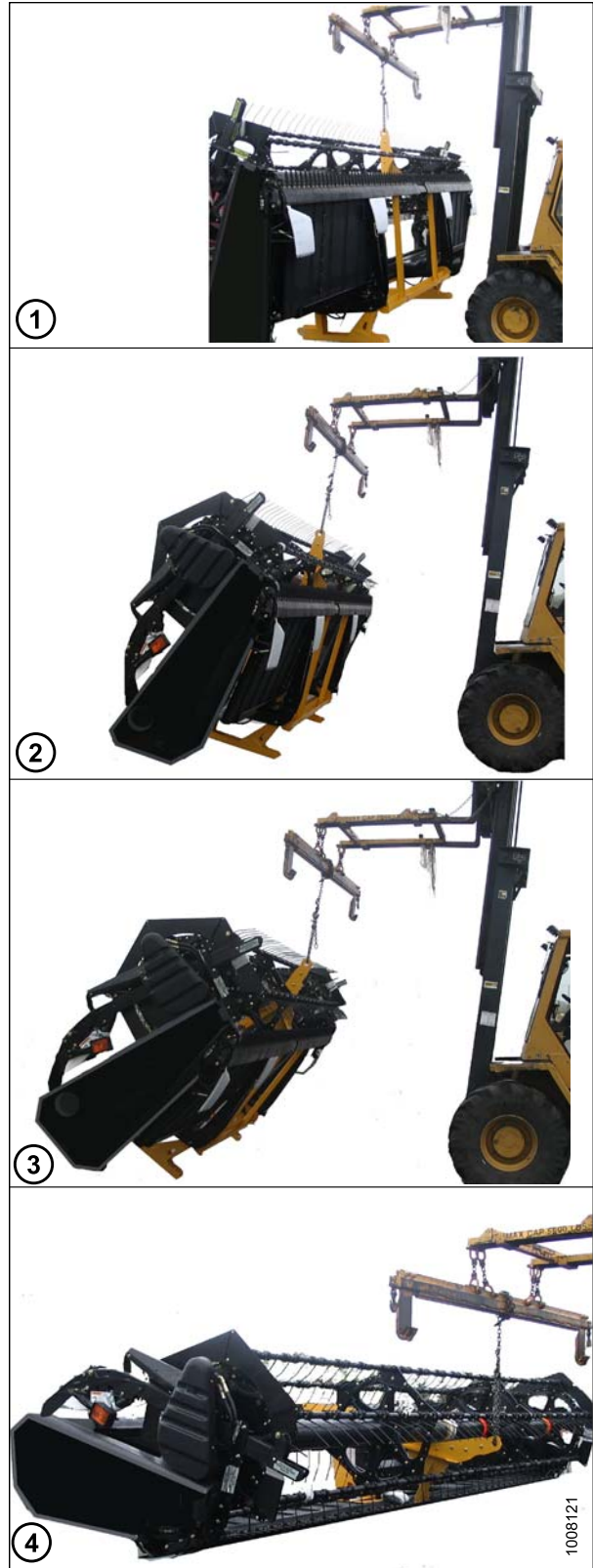
Figure 2.6: Header Lowered onto Ground
