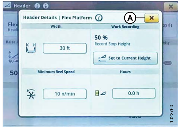
Figure 7.281: John Deere S7 Display – Header Details Window
