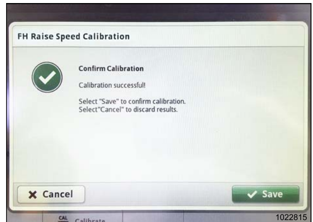
Figure 7.299: John Deere S7 Display – Feeder House Calibration
