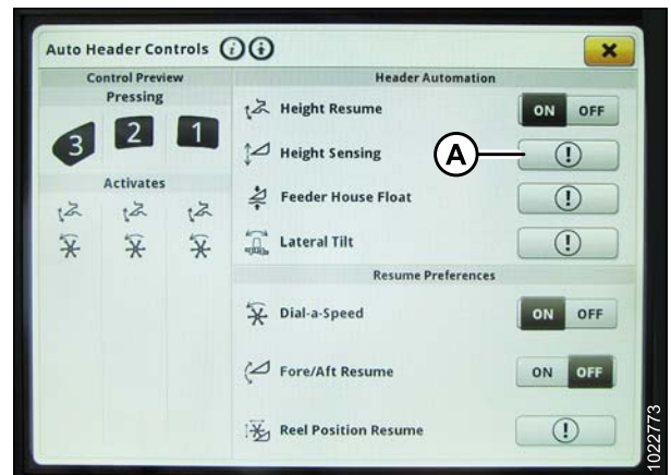
Figure 7.285: John Deere S7 Display – Auto Header Controls
