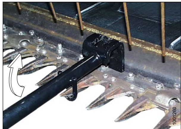
Figure 9.7: Straightening Tool – Upward Adjustment
