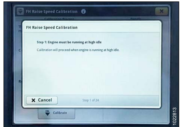
Figure 7.298: John Deere S7 Display – Feeder House Calibration
