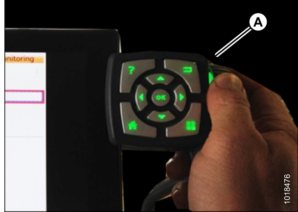
Figure 7.202: Adjustment Wheel on Right Side of Tyton Terminal
