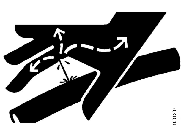
Figure 1.9: Hydraulic Pressure Hazard
