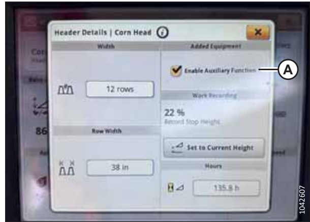
Figure 6.3: John Deere Combine Display – Header Details Dialog Box
