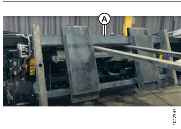
Figure 4.14: Removing Header Stand
