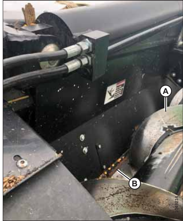
Figure 5.14: Auger-to-Stripper Bar Clearance
