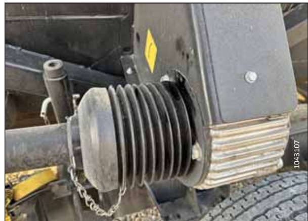
Figure 3.2: Main Driveline Guard – Correctly Seated
