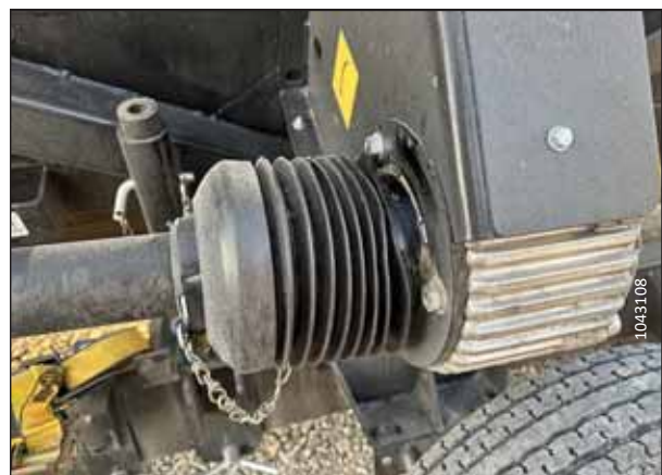
Figure 3.3: Main Driveline Guard – Incorrectly Seated
