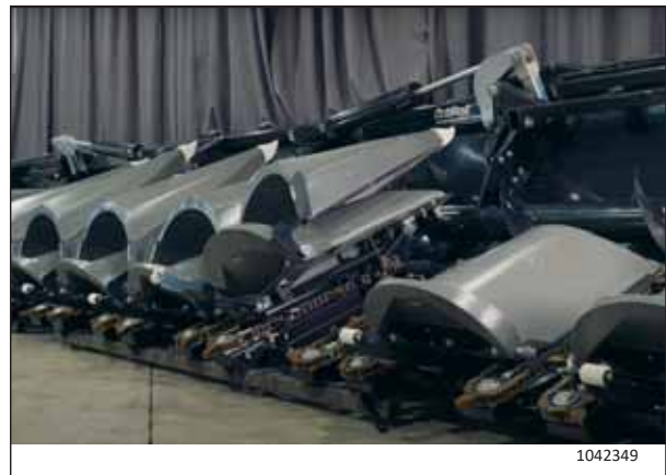
Figure 4.41: Snouts in Shipping Position
