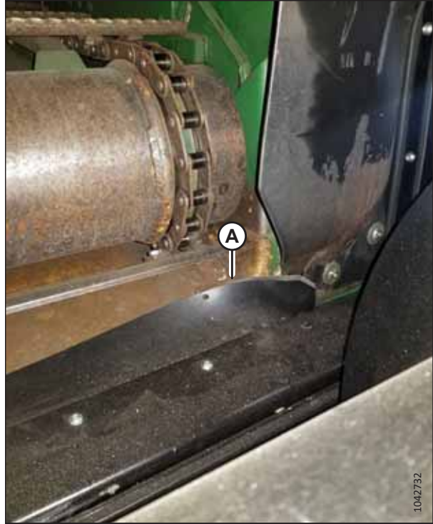
Figure 4.18: Too Large Transition Frame Seal
