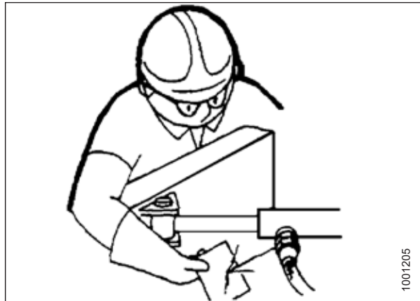
Figure 1.8: Testing for Hydraulic Leaks
