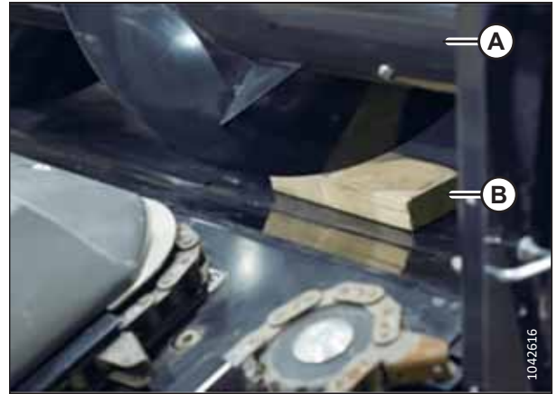
Figure 5.12: Auger Resting on Wood Block
