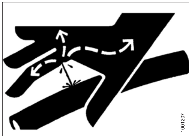
Figure 1.9: Hydraulic Pressure Hazard
