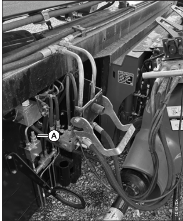
Figure 8.6: Pressure Relief Valve Adjuster Screw
