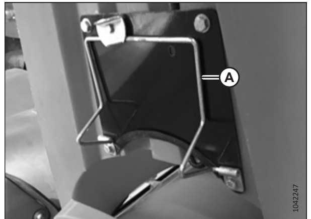
Figure 4.43: Wire Bracket Support Installed on Front Snout – Field Position
