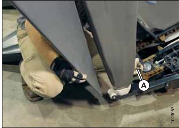
Figure 4.38: TED Installed on Left Standard End Divider
