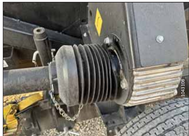
Figure 3.12: Main Driveline Guard – Incorrectly Seated
