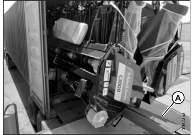
Figure 3.4: Removing Header Cart from Container
