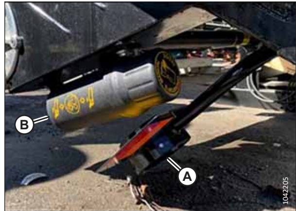
Figure 3.6: Clearance Light – Incorrect Position
