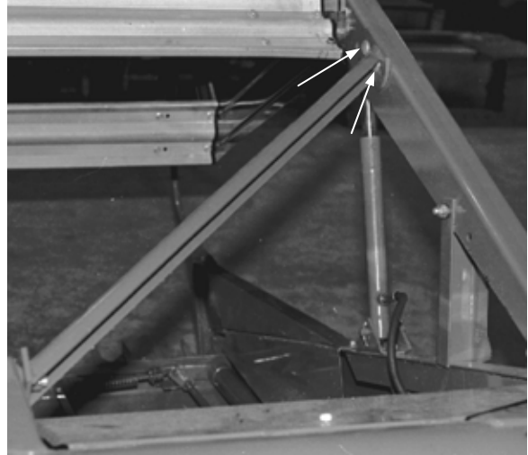
ADJUST BRACE TO CENTER REEL 496
