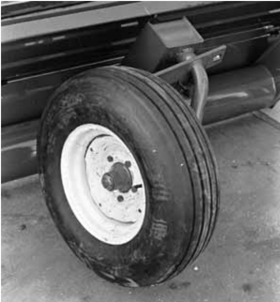
INSTALL R/H WHEEL 404
