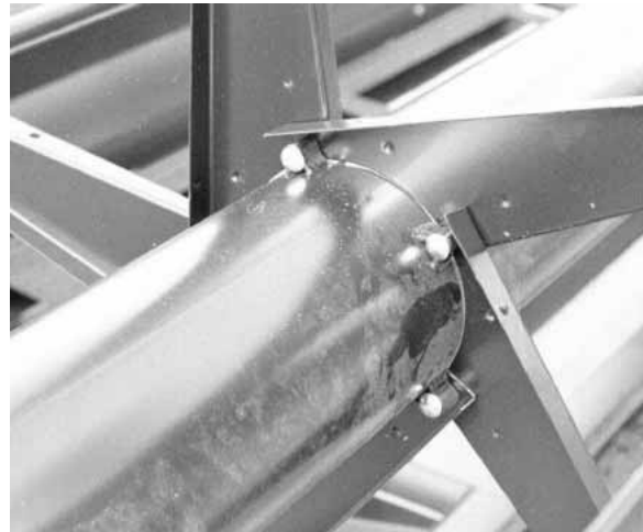
FASTEN REEL ARMS TO MAIN TUBE
