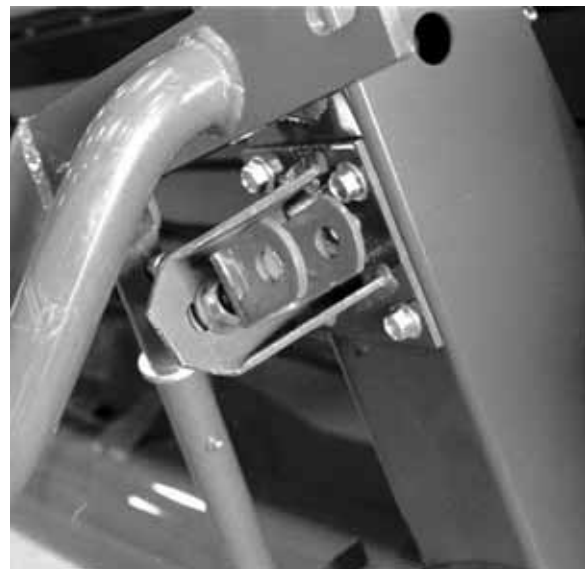
ATTACH CLEVIS TO R/H WHEEL 405
