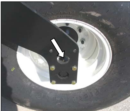
FORKED CASTER SPINDLE BEARINGS TWO PLACES (BOTH WHEELS)
