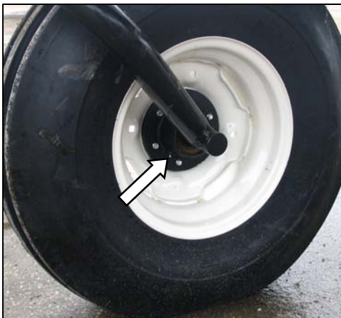
FORMED CASTER WHEEL BEARING 1 PLACE (BOTH WHEELS)
