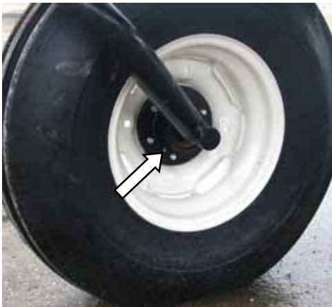
FORMED CASTER WHEEL BEARING 1 PLACE (BOTH WHEELS)
