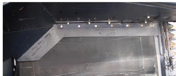
DEFLECTOR AFTER TRIMMING
