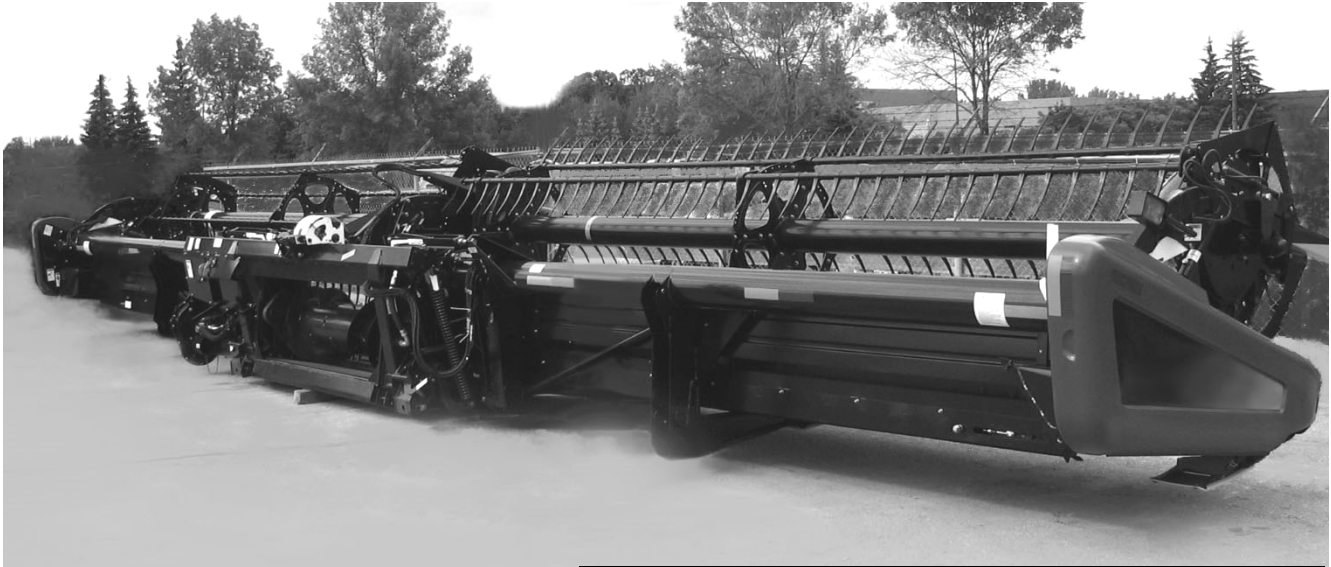
MacDon FD70 FlexDraper with CA20 Combine Adapter
