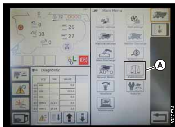
Figure 8.259: Menu d'étalonnage direct
