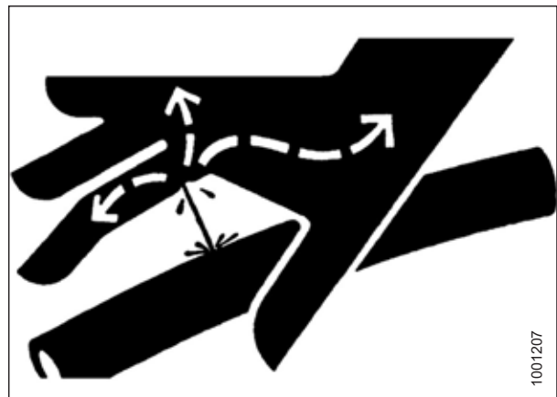
Figure 1.9: Hydraulic Pressure Hazard
