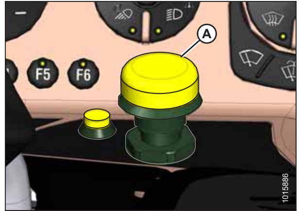
Figure 5.16: Header Engage Switch
