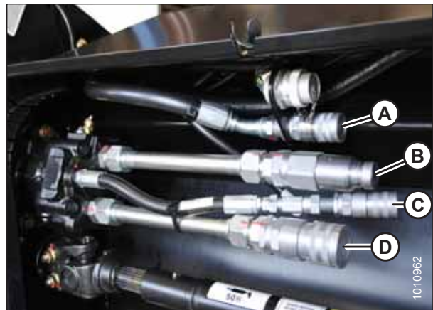
Figure 3.52: A40D Hose Connections – 5.4 m (18 ft.) Header Shown
