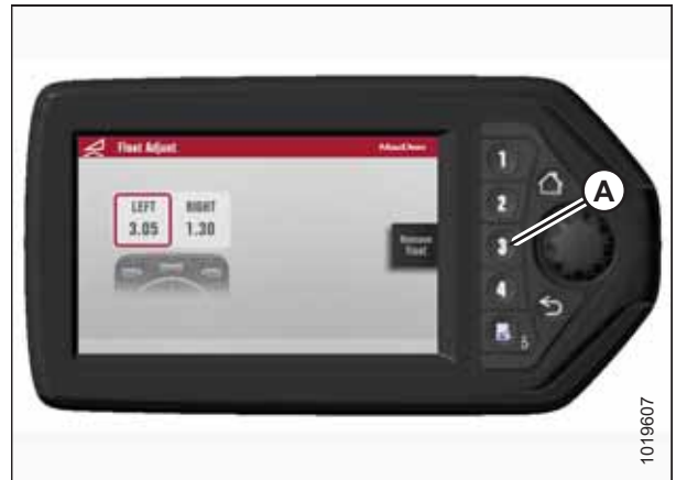
Figure 5.12: HPT Display – Adjusting Float
