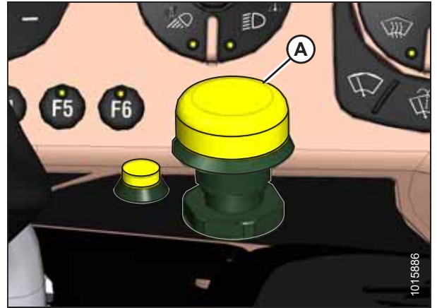
Figure 5.28: Header Engage Switch
