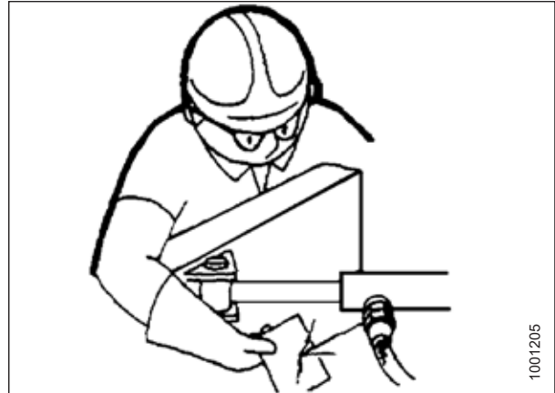
Figure 1.8: Testing for Hydraulic Leaks
