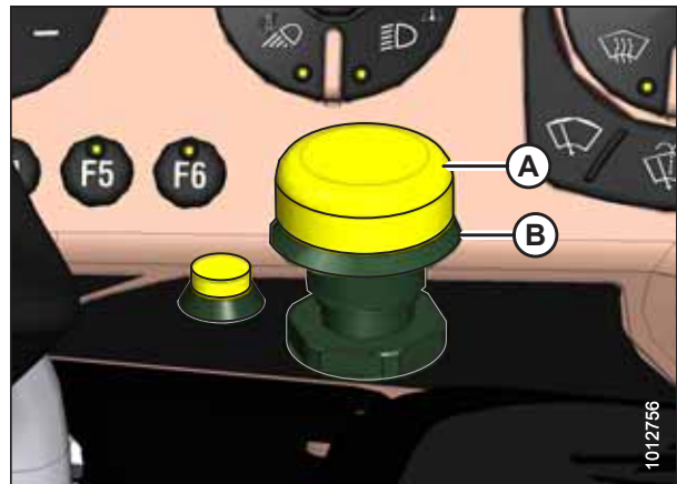
Figure 5.14: Header Engage Switch
