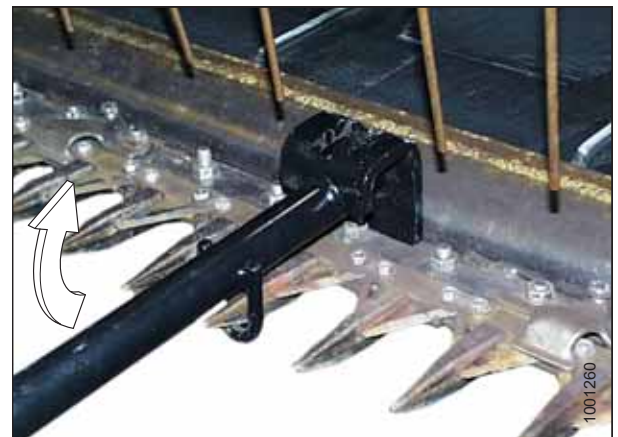
Figure 5.70: Guard Tips – Upward Adjustment
