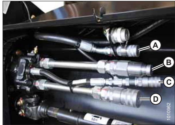
Figure 3.66: A40D Hose Connections – 5.4 m (18 ft.) Header Shown
