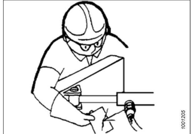
Figure 1.8: Test de fuites hydrauliques
