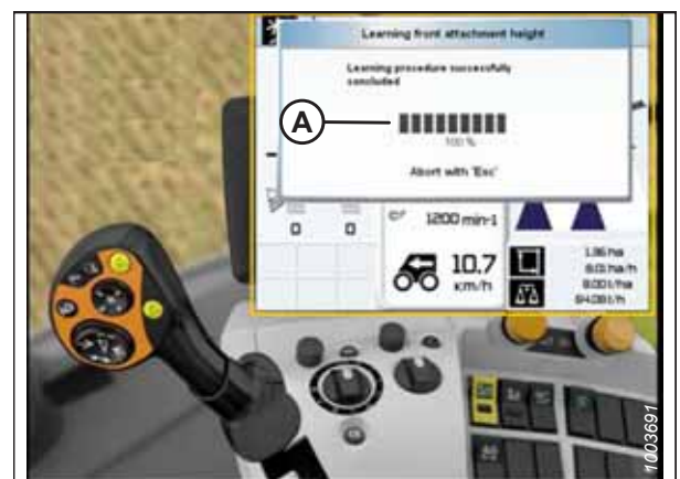
Figure 8.137: CLAAS Lexion Combine Display, Console, and Control Handle
