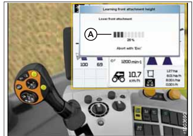
Figure 8.136: CLAAS Lexion Combine Display, Console, and Control Handle
