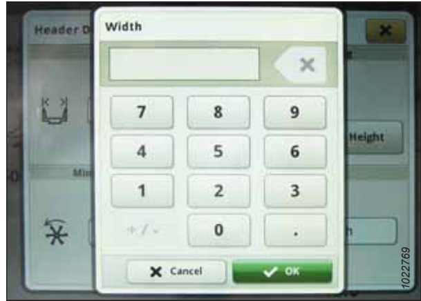
Figure 8.350: John Deere S7 Display – Setting Header Width
