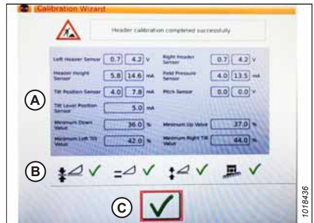
Figure 8.225: Completed Calibration Page
