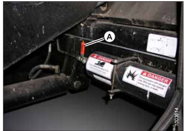
Figure 8.190: Combine Accumulator ON/OFF Switch A - Accumulator Lever (Off Position)
