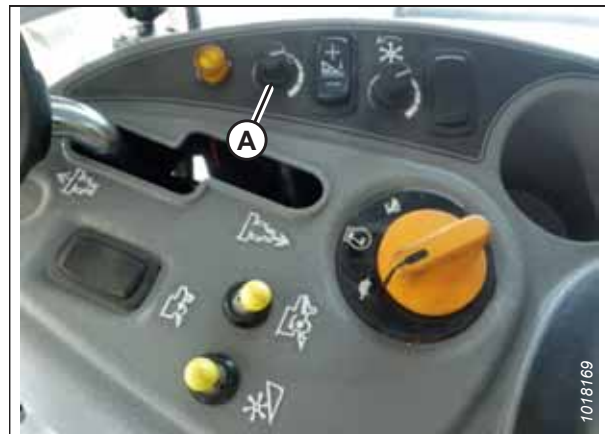
Figure 8.102: Height Adjustment Knob on the Combine Control Console
