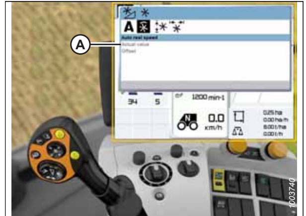
Figure 8.144: CLAAS Lexion Combine Display, Console, and Control Handle
