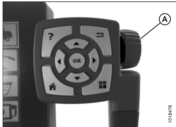
Figure 8.232: Adjustment Wheel on Right Side of Tyton Terminal
