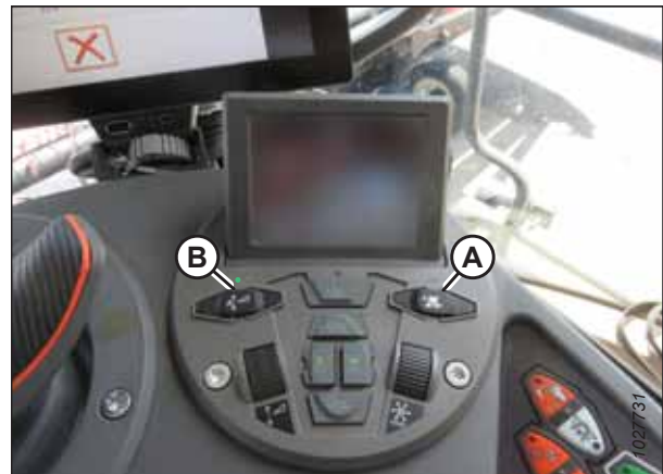
Figure 8.261: Header Control Cluster
