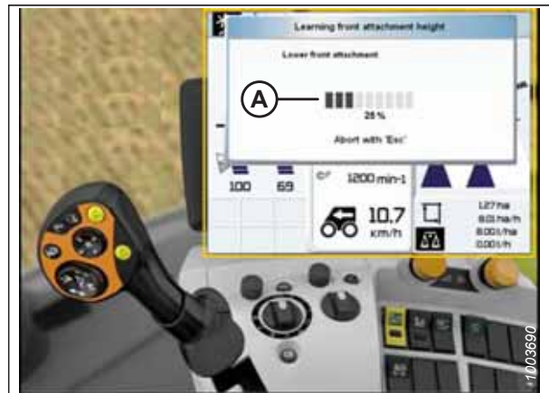
Figure 8.151: CLAAS Lexion Combine Display, Console, and Control Handle
