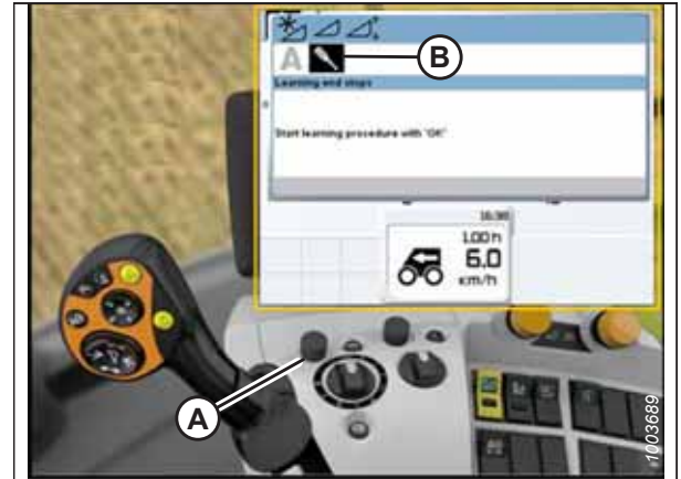
Figure 8.135: CLAAS Lexion Combine Display, Console, and Control Handle
