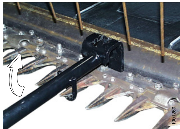
Figure 8.7: Guard Tips – Upward Adjustment
