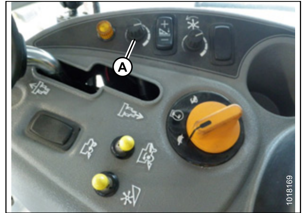
Figure 6.59: Height Adjustment Knob on the Combine Control Console
