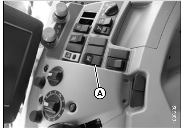
Figure 4.79: Switch in Console
