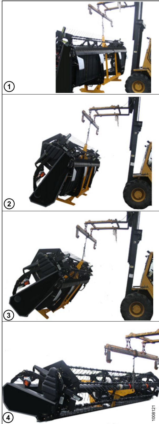
Figure 2.6: Header Lowered onto Ground
