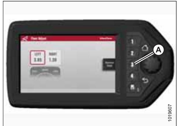
Figure 5.12: HPT Display – Adjusting Float
