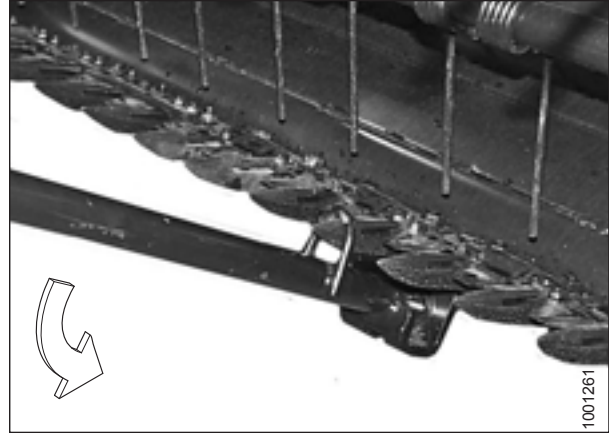
Figure 5.42: Guard Tips – Downward Adjustment
