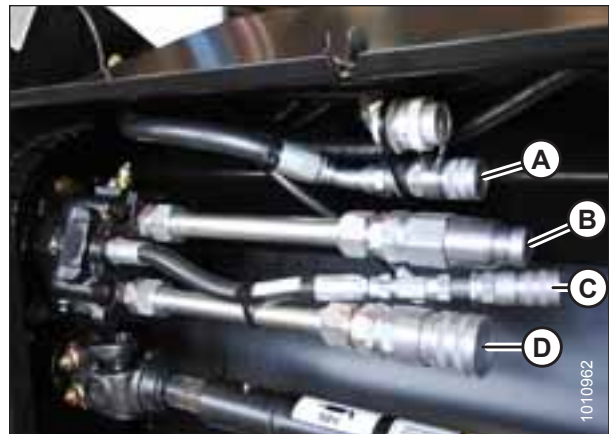
Figure 3.64: A40D Hose Connections – 5.4 m (18 ft.) Header Shown
