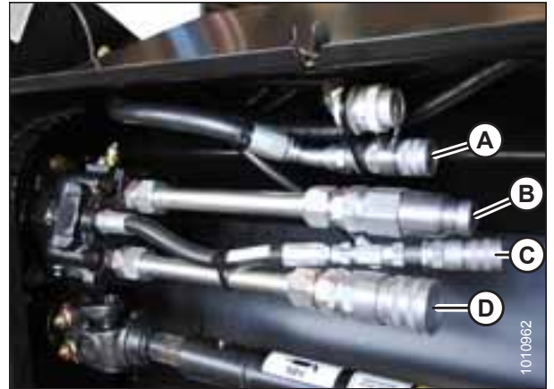
Figure 3.51: A40D Hose Connections – 5.4 m (18 ft.) Header Shown
