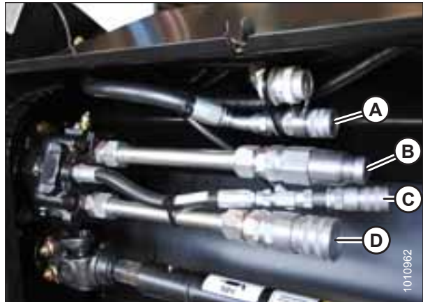
Figure 3.93: A40D Hose Connections – 5.4 m (18 ft.) Header Shown
