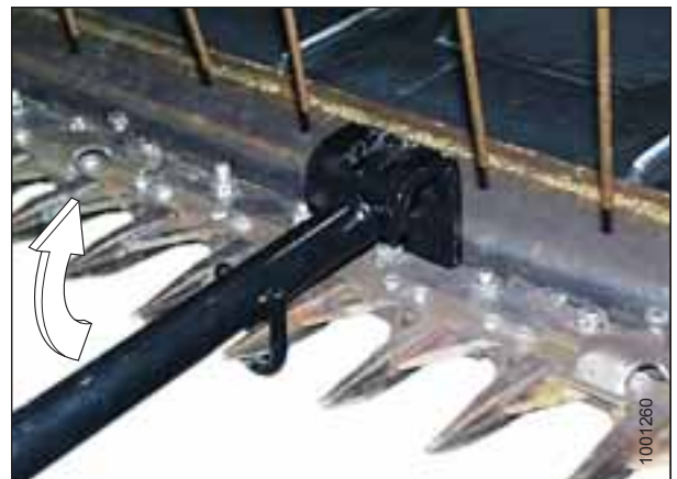
Figure 5.41: Guard Tips – Upward Adjustment
