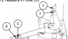
☐ If mounting adapter to a 974/84C header, move down stop pad to outboard set of holes (both sides) as shown.
