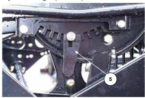
☐ Set the fore/aft position to between **4** and **5** on the gauge decal at left reel support arms.
