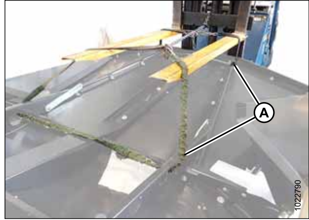
Figure 2.9: Lifting Forming Shield with Forklift
