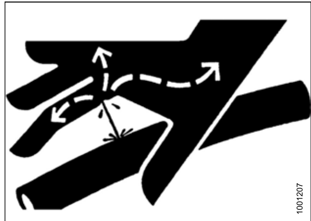
Figure 1.12: Hydraulic Pressure Hazard
