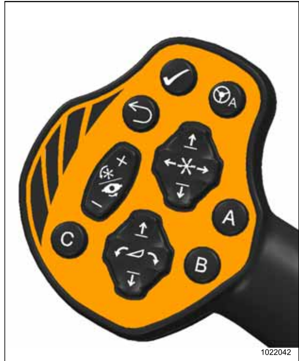
Figure 3.11: Ground Speed Lever (GSL)
