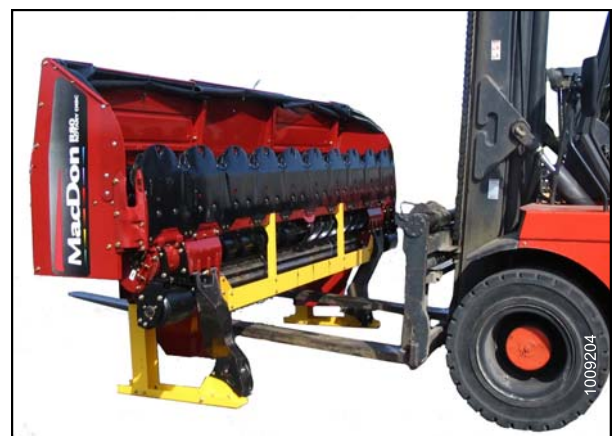
Figure 2.2: Moving Header with Forklift
