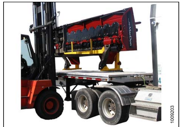
Figure 2.1: Lifting Header off Trailer
