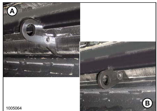
Figure 4.15: Roll Timing Gauge in Use
