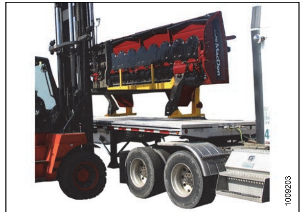
Figure 2.1: Lifting Header off Trailer
