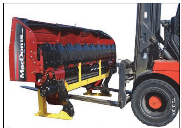
Figure 2.2: Moving Header with Forklift
