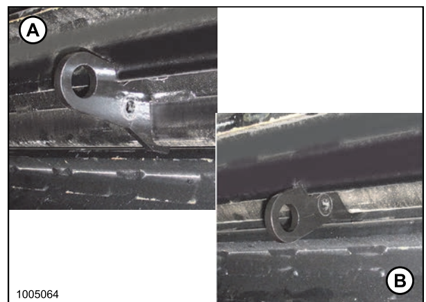
Figure 4.15: Roll Timing Gauge in Use
