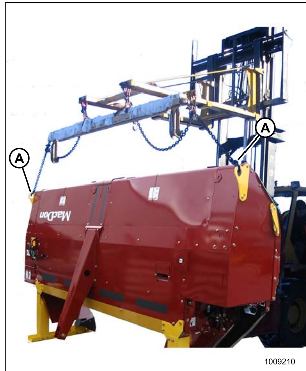
Figure 3.3: Spreader Bar Attached to Header
