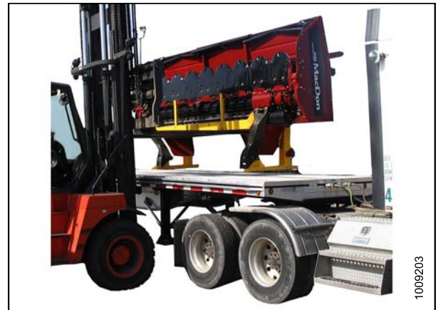
Figure 5.1: Lifting Header off Trailer
