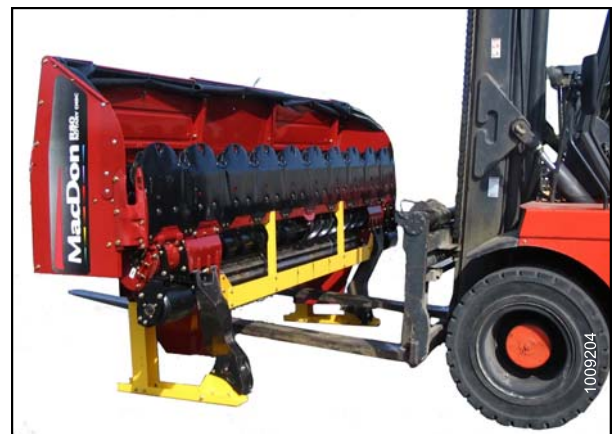
Figure 5.2: Moving Header with Forklift
