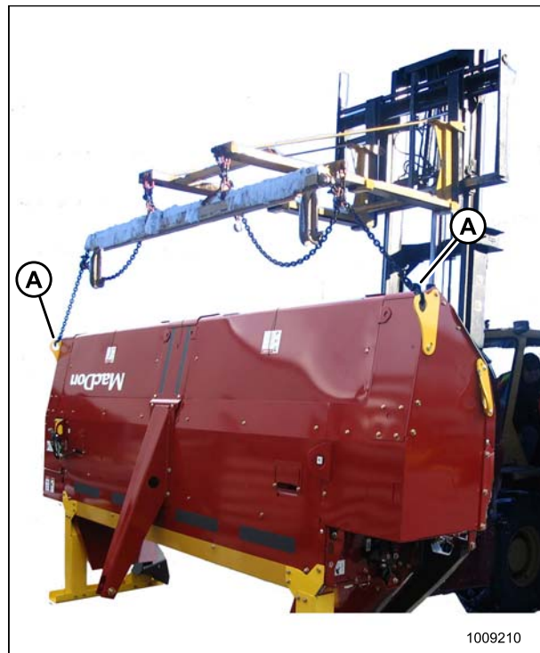
Figure 6.3: Spreader Bar Attached to Header
