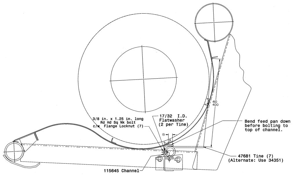
NOTE: For all 910 and 920 headers up to S/N 86399, modify conditioner feed pan by cutting at rear to dimension 19 as shown.
