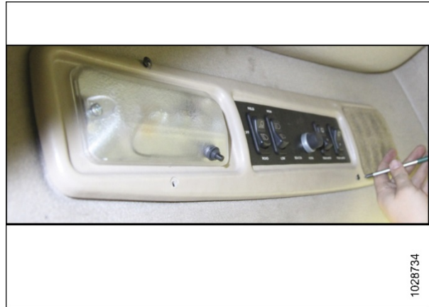
Figure 14: Right Headliner Switch Panel
