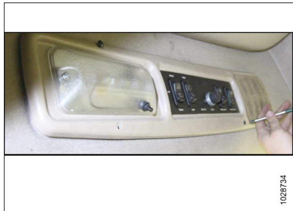
Figure 2: Right Headliner Switch Panel
