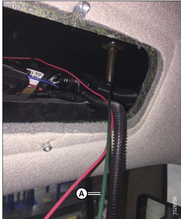
Figure 5: Routing Stiff Wire Through Opening in Headliner
