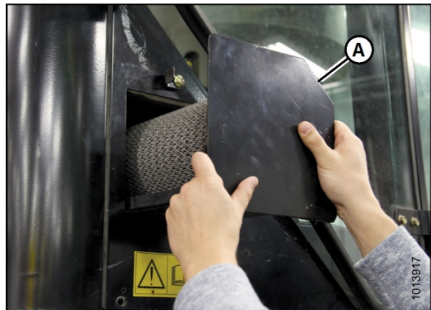
Figure 13: Reinstalling Air Filter Pan and Filter
