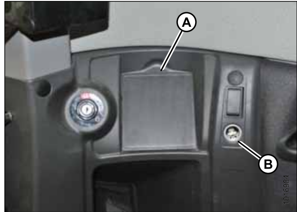
Figure 3.47: Access Panel beside Ignition
