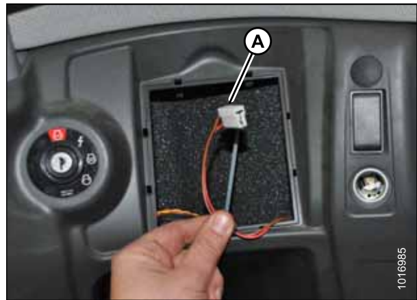
Figure 3.48: Switched Power Harness Plug
