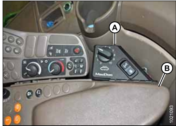
Figure 3.19: Control Panel Installed
