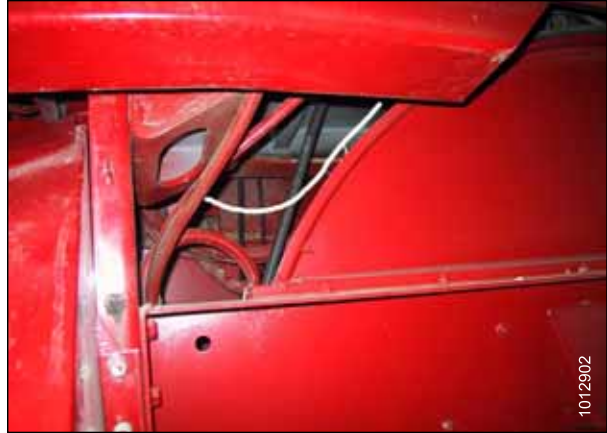
Figure 3.28: Harness Routing over Combine Rotor
