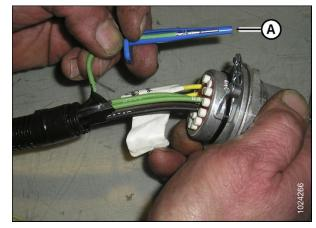
Figure 6: Pulling the Wire
