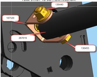
ATTACH NEW TUBE STRUT 287619 SUPPLIED IN KIT. REUSE 136455 BOLT AND 136440 NUT TO CONNECT TUBE STRUT TO BOTTOM ANCHOR.
