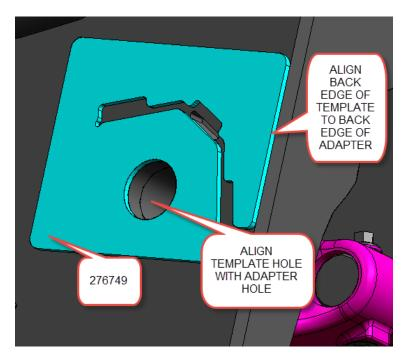
USING TEMPLATE TO POSITION 295333 GUIDE, NOTE THAT TEMPLATE 276749 IS A LOCATING TEMPLATE ONLY. WELD GUIDE TO SIDE OF ADAPTER FRAME WITH THE THREE WELDS INDICATED BELOW. TEMPLATE HAS NOTCHES SHOWING POSITION OF THE THREE WELDS. SUGGEST TACK WELDING 295333 AT BOTTOM RIGHT CORNER PRIOR TO REMOVING TEMPLATE. REMOVE TEMPLATE BEFORE WELDING GUIDE TO ADAPTER FRAME.
