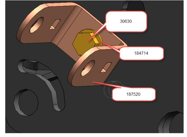
THEN USING EXISTING ANCHOR 187520 REATTACH TO THE NEW THREADED HOLE POSITION USING 30630 BOLT (M12X1.75X 30) AND FLAT WASHER 184714. ORIENTATE THE ANCHOR AS SHOWN BELOW.
