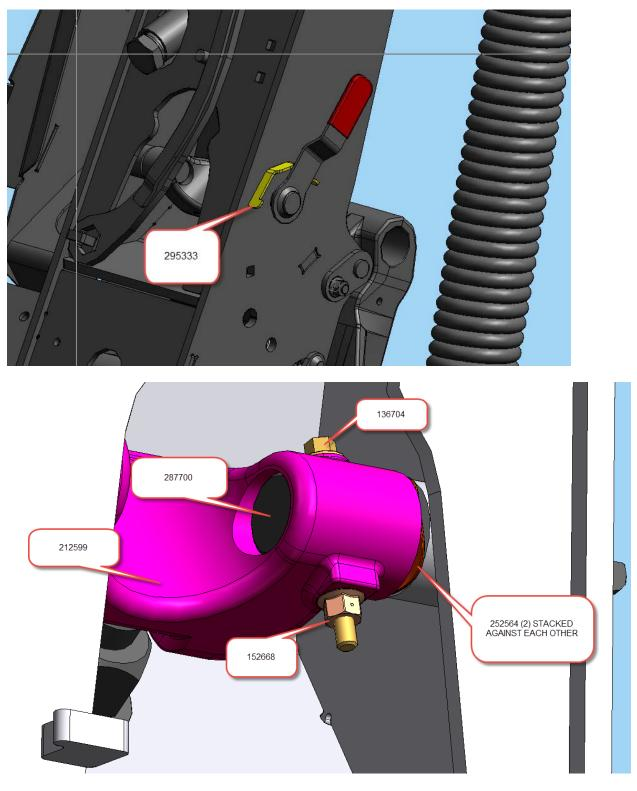
E) TO SLOW DOWN TILT CYLINDER SPEED WE REQUIRE 252692 RESTRICTOR TO BE ADDED TO HYDRAULIC TOP LINK ASSEMBLY. THREAD 252692 RESTRICTOR INTO ROD END PORT OF CYLINDER UNDER ELBOW FITTING.
