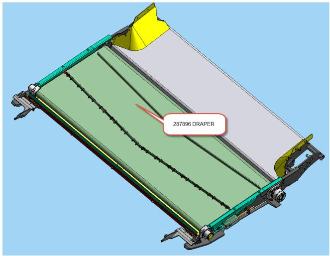
THE LH AND RH GUIDE –IDLER ADJUSTMENT NEED CHANGED TO THE NEW 287677 AND 287678 SUPPLIED IN KIT. THE COMPRESSION SPRINGS NEED CHANGED TO THE NEW 287587 SPRINGS. THE IDLER CUP ASSEMBLIES 248738, 248740 NEED TO BE CHANGED TO THE NEW 287885 AND 287883 IDLER CUP ASSEMBLIES.
