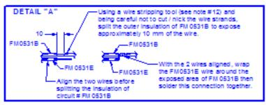
10. After the solder connection has cooled, re-position the heat shrink over the splice (centered) then apply heat to the tubing to shrink it down over the wires / splice and seal the connection.
