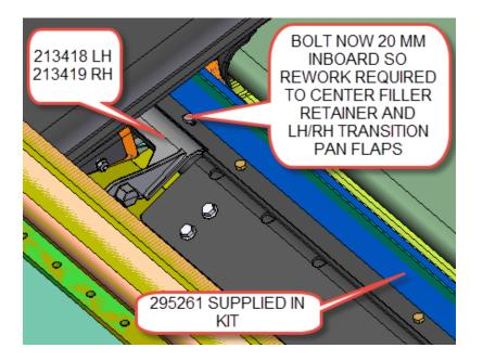
REWORK EXISTING CENTER FILLER RETAINER 213236 INTO 287778 BY DRILLING TWO HOLES AS SHOWN BELOW. OTHER OPTION INSTEAD OF HOLES IS TO LENGTHEN EXISTING SLOTS BY 13 MM .
