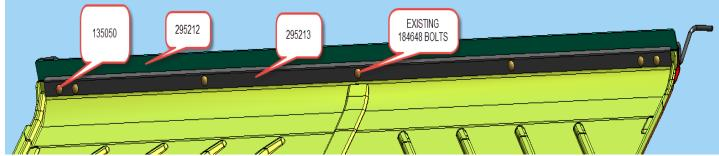
TIGHTEN THE THREE 135337 NUTS ON 184648 BOLTS TO 150 IN LBS.
