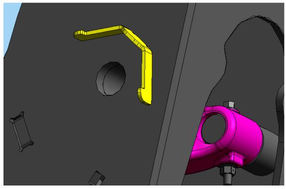
ASSEMBLE NEW HANDLE ASSEMBLY 287700 SUPPLIED IN KIT AS SHOWN BELOW. ASSEMBLE WAVE WASHERS 252564 (2) (STACKED AGAINST EACH OTHER) SUPPLIED IN KIT BETWEEN TUBE (WELDED TO INSIDE OF FRAME) AND 212599 DOWNSTOP CASTING.
