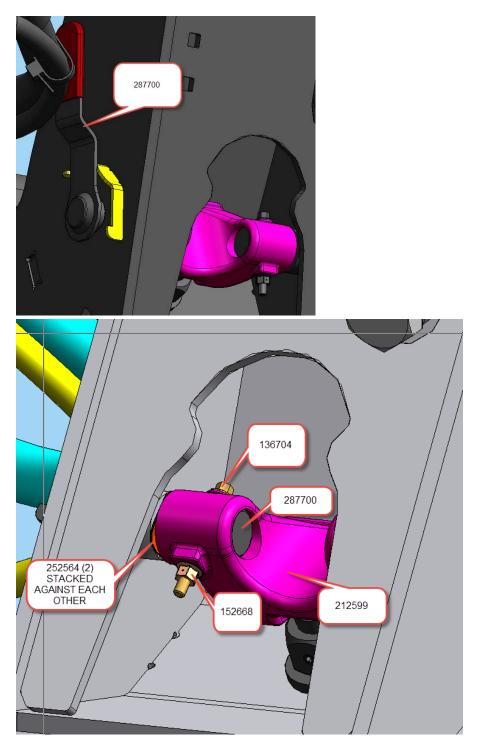
REPEAT ABOVE PROCEDURE TO WELD ON FLOAT LOCK GUIDE 295333 TO THE RIGHT SIDE OF THE ADAPTER AS SHOWN BELOW. REPLACE RH PIVOT SHAFT WELDMENT 240247 WITH 287700 HANDLE ASSEMBLY. WAVE WASHERS 252564 (2) (STACKED AGAINST EACH OTHER) BETWEEN WELDED TUBE AND 212599.
