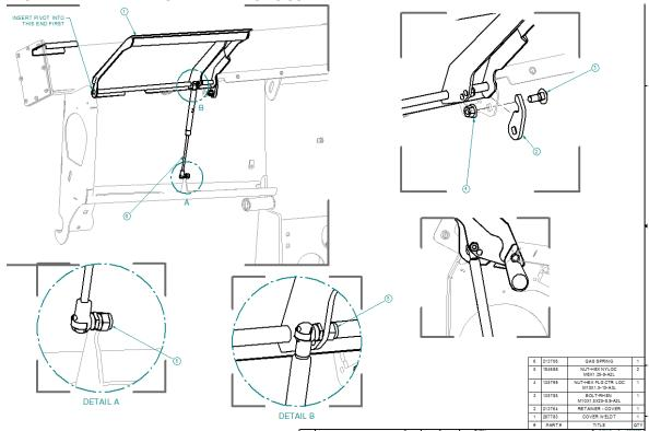
C) THE GEARBOX STRUT ANCHOR NEEDS TO BE RELOCATED. REMOVE OLD TUBE STRUT AND ANCHOR FROM ADAPTER FRAME. LEAVE ANCHOR AT GEARBOX AS IS. USING 287620 TEMPLATE SUPPLIED IN KIT, POSITION IT AS SHOWN ON ADAPTER FRAME.
