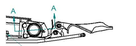
INSTALL NEW FEED DRAPER AROUND REAR DRIVE ROLLER BEFORE YOU INSTALL FRONT IDLER ROLLER. ONCE FEED DRAPER IS BOLTED TOGETHER SLIDE IDLER ROLLER WITH NEW CASTINGS THROUGHDRAPER. ATTACH NEW IDLER GUIDES 287677 AND 287678 TO IDLER CASTING AND PLACE IN FRAMES. APPLY ABOUT 125 GRAMS OF TALCUM POWDER TO INSIDE OF FEED DRAPER. APPLY LIBERALLY TO "V" GUIDE AREA AND ACROSS ENTIRE WIDTH. INSTALL WITH EXISTING CONNECTORS AND HARDWARE. NOTE THAT CHEVRON CLEATS ON TOP MUST POINT TOWARDS FRONT.
