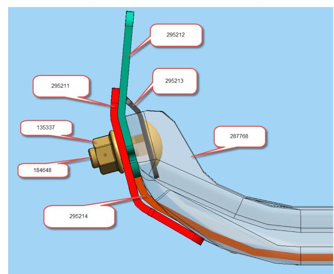
H) THE FOLLOWING INVOLVES CHANGES TO FEED DECK ASSEMBLY. REMOVE EXISTING DRAPER FROM DECK ASSEMBLY.
