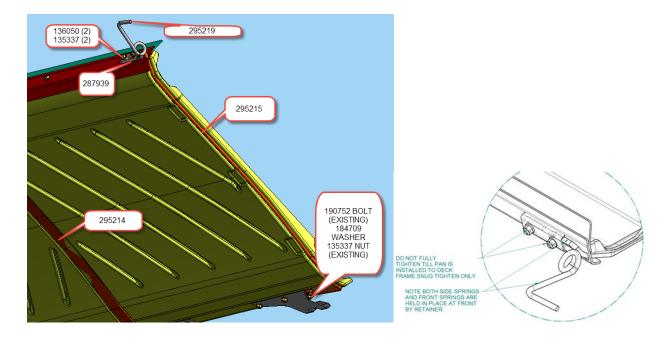
NOTE THAT WASHER 184709 SUPPLIED IN KIT GOES BETWEEN 135337 NUT AND 295215, 295216 SIDE SPRING AT THE REAR CONNECTION. LINE UP FRONT BAR OUTER PLATE 295211 WITH POLY PAN AND DRILL HOLES OUT IN POLY PAN.
