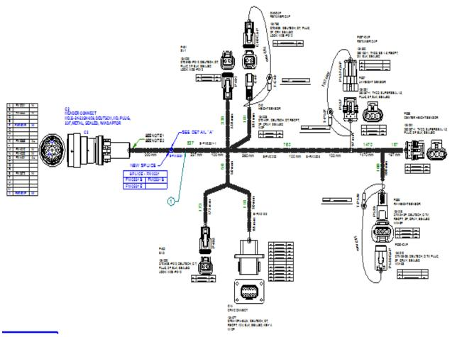
PARTS REQUIRED FOR HARNESS REWORK INCLUDE 291277 WIRE, 134013 CONTACT REMOVAL TOOL AND HEAT SHRINK TUBE 186161. ALL THESE PARTS INCLUDED IN KIT.
