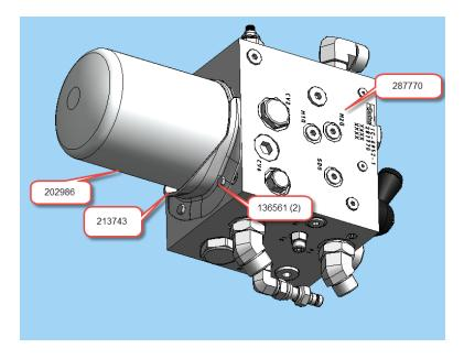
Change hoses 213240, 213242 to 287907 (2), 213241 to 287908, 213248 to 287910 and 213245 to 287909. Put same color cable tie to same location on replacement hoses. Assembly to manifold to be as shown in below images. Add the three 135444 cinch straps around the five hoses as shown below.
