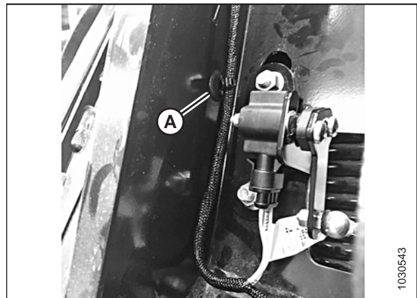
Figure 3.15: Securing Right Sensor Harness
