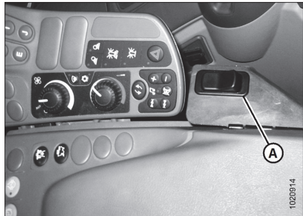
Figure 1: Reel Fore-Aft / Header Tilt Selector Switch in John Deere Combine Cab (Position of Switch is Similar in Challenger, Gleaner, and Massey Ferguson Combine Cabs)
