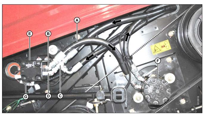
Figure 3.8: New Reel Motor, Auger Motor, Hoses, and Fittings (M100, M105, M205 Configuration)
