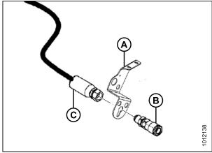
Figure 3.16: 16-Foot Grass Seed Header – End of Reel Drive Case Drain Hose (Windrower Case Drain Hose Not Shown)
