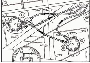
Figure 3.3: Hydraulic Line Configuration for Previous Reel Motor (MD #124096) for M100, M105 or M205
