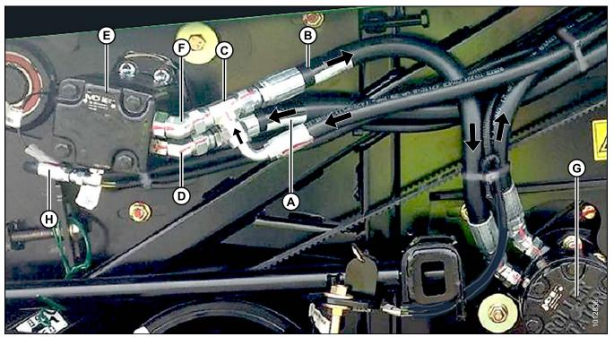
Figure 3.12: New Reel Motor, Auger Motor, Hoses, and Fittings (M150, M155, M200 Configuration)
