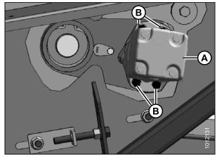
Figure 3.11: New Motor Assembly Installed
