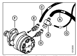
Figure 3.9: Previous Reel Motor MD #124096 with Hoses and Fittings (Shown in Factory Configuration for M150, M155 or M200)
