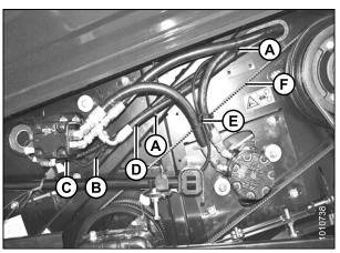
Figure 3.18: Cable Tie Locations (M205 Configuration Shown – M155 Uses Same Locations)
