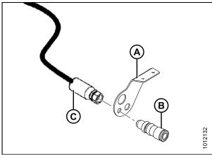
Figure 3.15: 14-Foot Grass Seed Header – End of Reel Drive Case Drain Hose (Windrower Case Drain Hose Not Shown)
