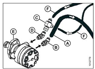
Figure 3.5: Previous Reel Motor MD #124096 with Hoses and Fittings (Shown as Configured for M100, M105 or M205)
