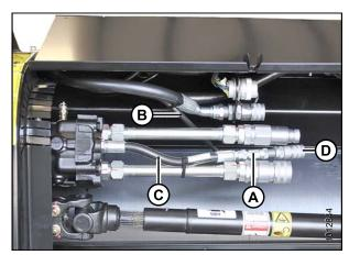
Figure 3.14: Knife Drive Motor Connections on 18-Foot Non Grass Seed Header (Other Hoses Not Shown)
