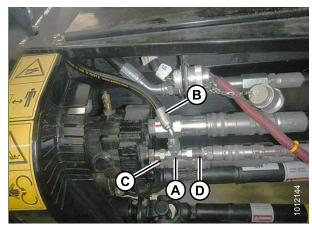
Figure 3.13: Knife Drive Motor Connections on 14- or 16-Foot Non Grass Seed Header
