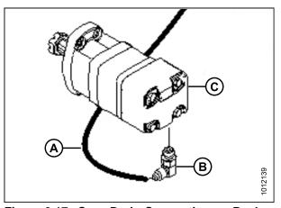
Figure 3.17: Case Drain Connection on Reel Drive Motor (Other Hoses Not Shown)
