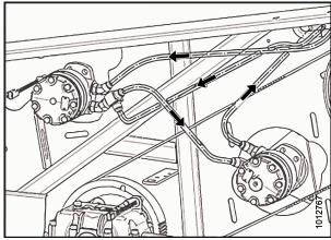
Figure 3.4: Hydraulic Line Configuration for Previous Reel Motor (MD #124096) for M150, M155 or M200
