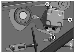
Figure 3.7: New Motor Assembly Installed
