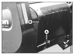
Figure 3.2: Driveline Shield
