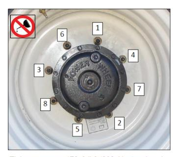
Tighten nuts to 170 ft·lbf (230 N·m) using the tightening sequence as shown above.
