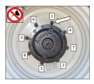
g. Install L9 nuts and L9 washers, and tighten to 170 ft·lbf (230 N·m) using the tightening sequence as shown above.
