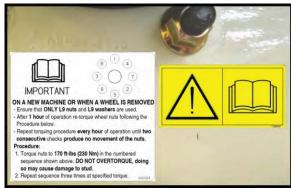
Figure 5 – New Drive Wheel Decal MD #166584 And READ MANUAL Decal MD #166454
