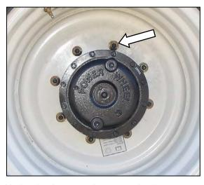
e. Undo wheel nuts, and remove wheel.
