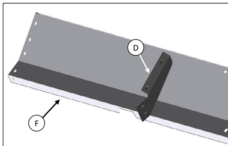
3. Sandwich the tabs on the shield extension provided in the kit (G) in between the new shield provided in the kit (F) and the existing conditioner covers (H) installed on the header. Attach with two of the carriage bolts (J) and flange nuts included in the kit.
