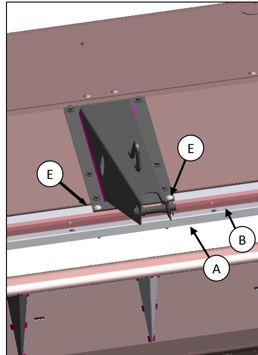
2. Attach right- and left-hand conditioner cover angles (D) to the conditioner shield (F) provided in the kit using the hardware removed in step 1. d.
