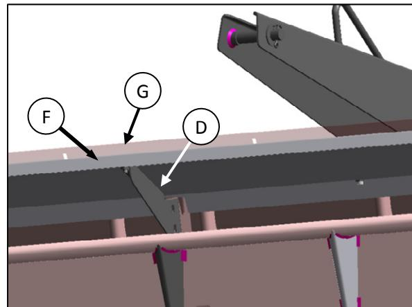
5. Connect center tower to the new conditioner shield (F) using the bolts already in place (E).
