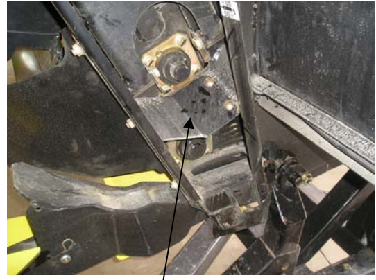
Remove deflector at RH header leg
