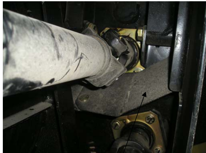
Remove deflector at RH header leg
