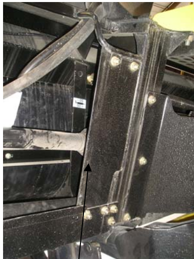
Remove shield at LH header leg
