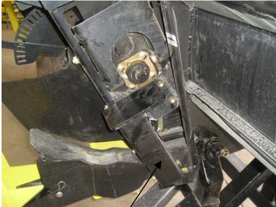
Remove jack at RH header leg
