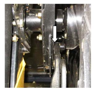
Sufficient clearance between the cam arms and cam disc must be maintained to prevent the cam arms from contacting the cam disc during operation. If contact is evident, the cam disc should be re-aligned and/or the clearance between the cam arms and cam disc should be adjusted.
