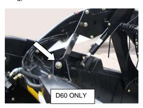
c. Remove bolt in LH reel arm brace so that reel arm is free to move when removing the reel.
