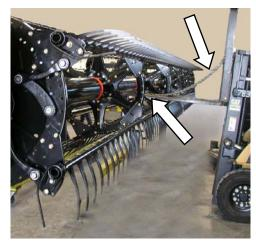
Locate forks under reel tube at approximately the center disc and secure tube to forklift with a chain, OR locate a sling around reel tube and attach to a forklift or equivalent (See B DOUBLE REEL HEADERS).
