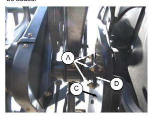
b. Loosen four nuts (A) on cam disc.
