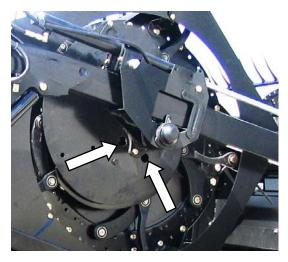
d. At cam end, rotate reel to line up bolts attaching cam hub to reel tube with access holes in cam disc. This allows access to the bolts with a socket and extension.
