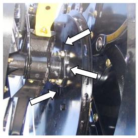
d. At cam end, rotate reel to line up bolts attaching cam hub to reel tube with access holes in cam disc. This allows access to the bolts with a socket and extension.
