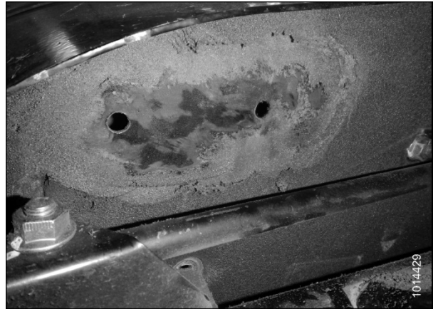
Figure 4: Foam Removed from Windrower Cab
